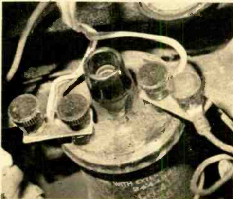
Pre-wired ignition-coil terminal boards fit on coil screws. Thumb nuts come with kit and allow you to switch back to original ignition system.
