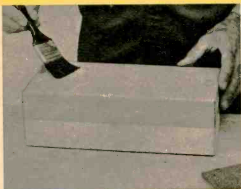
Fig. 3—Using an ordinary paint brush, apply the resin to the box or whatever form you are going to use. Be sure you don't brush resin too thin.
