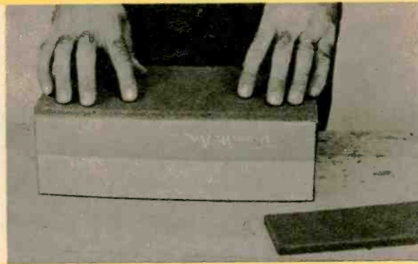
Fig. 4—After giving the box a coat of resin, give each of the pieces of Plyfoam a coat of resin. Then assemble the individual pieces on the box.
