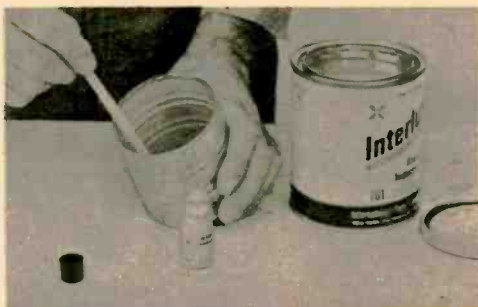
Fig. 2—Batch of polyester resin is prepared with hardener which produces a quick cure. Resin is interlux No. 701. Mixing instructions are on the can.
