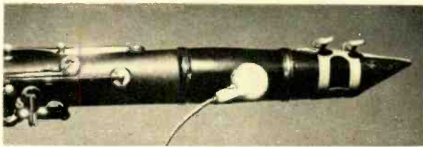
Fig. 1—Conn pickup mike (above) is installed in clarinet. Multi-Vider (right) clips on belt. Two top switches (at left of unit) boost or attenuate treble. Third switch from top adds octave above fundamental. Switch below adds one octave below fundamental. Fifth switch down adds second octave below fundamental. Bottom switch controls power. Top knob sets instrument's basic volume. Other controls set level of added octaves. Solid-state circuitry includes filters and frequency dividers. Unit is powered by 9-V battery and its output can be fed to any high-power musical-instrument amplifier.
