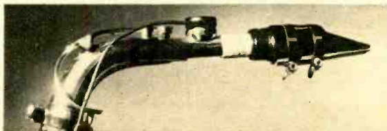
Fig. 2—Selmer pickup mike is installed in sax's neck (above). Control unit (right) is installed permanently on this sax but can be clipped on belt or hung around neck. Top switch (on left of unit) boosts treble. Switch under it boosts level of instrument's normal sound. Next switch attenuates treble. Bottom switch turns on tremolo. Top knob is master volume, middle controls reverb, bottom sets level of octave below. Unit must be used with Selmer's amp.
