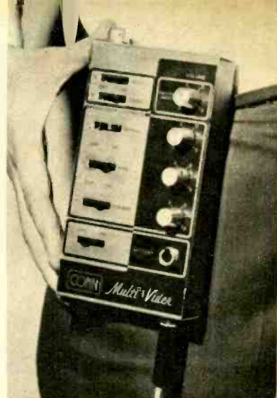
Fig. 1—Conn pickup mike (above) is installed in clarinet. Multi-Vider (right) clips on belt. Two top switches (at left of unit) boost or attenuate treble. Third switch from top adds octave above fundamental. Switch below adds one octave below fundamental. Fifth switch down adds second octave below fundamental. Bottom switch controls power. Top knob sets instrument's basic volume. Other controls set level of added octaves. Solid-state circuitry includes filters and frequency dividers. Unit is powered by 9-V battery and its output can be fed to any high-power musical-instrument amplifier.
