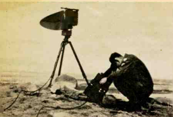
The Pipsy-Five (AN/PPS-5) still is undergoing tests at Ft. Huachuca. It produces a rough but useful TV-like picture of the area it surveys.
