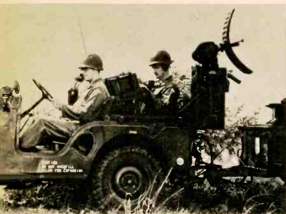
An AN/TPS-33 like this has foiled at least one recent Viet ambush. Pipsy-Four can also be Jeep-mounted but bouncing makes targets hard to spot.
