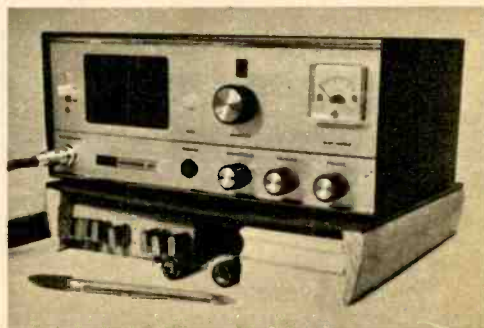
Top piece of CB rig's stand is same size as unit and is supported by two side pieces, somewhat higher in front than in back, to tilt set back.
