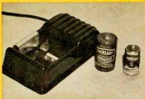
Rogers 880, available through parts distributors in blister pack, provided charging currents ranging from 500 ma for D cell to less than 1 ma per AA cell in Z battery. Circuit uses isolation transformer, silicon diode. Finger points to filter capacitor needed to control line hum for battery eliminator use.
