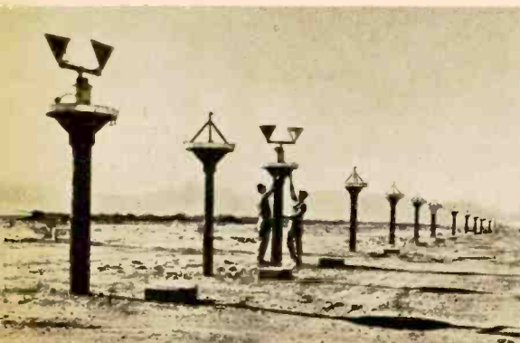
To check accuracy, radar is pointed at this radar spoke. Operators know precise spacing of posts, easily can spot inaccuracies or distortion.
