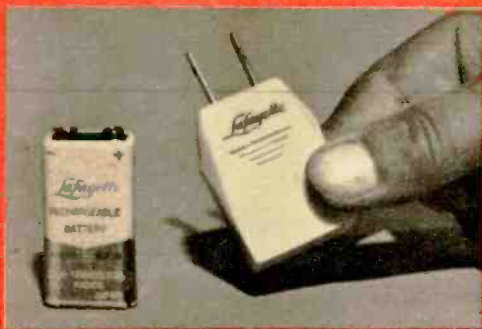
Combination rechargeable battery and plug-in charger, available from several mail-order houses, gave good results, can also be used with standard batteries. Charging circuit consists of series-connected resistor and selenium rectifier. Small resistor and neon lamp are only for ON indicator in this case.
