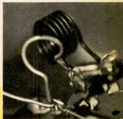
Fig. 2—Closeup of homebrew coils. L1 is at left. After making single turn, spread loop 5/16 in. Length of leads to switch lugs must be exactly 1/4 in. Coil L2, 5 closewound turns, also must be mounted no more or less than 1/4 in. from lugs on switch.
