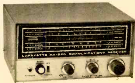
Fig. 1—Lafayette HA-226 short-wave receiver does not have bandspread and can use it. Control we added is at left between phone jack and switch.
