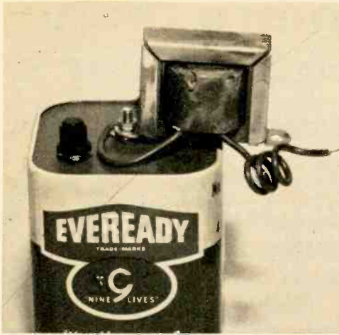
Power supply consists of 6-V battery in series with filament transformer's secondary. Mount transformer as shown to change battery easily.
