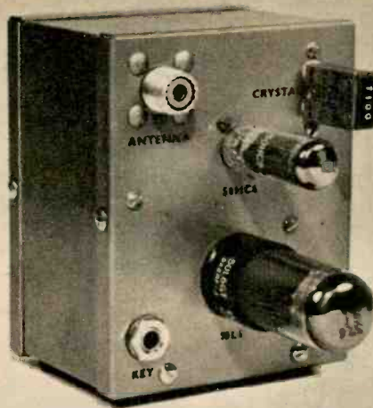
Fig. 7—Rear view of Mini-Mitter. If you feel uneasy about building the transmitter in such a small box the answer is obvious. Get a larger cabinet!
