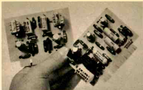
MAJORITY of KG-415 components are mounted on six printed-circuit modules similar to these two.
