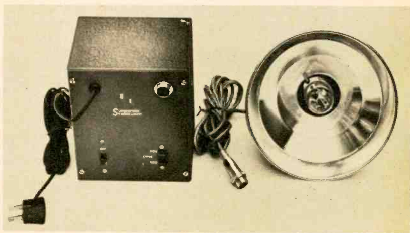
Fig. 1—Strobe consists of 4 x 5 x 6-in. power pack and 6 \frac{3}{4} -in.-dia. flash head. Flash head plugs in socket at top of power pack. Socket below is for sync cable to camera.
