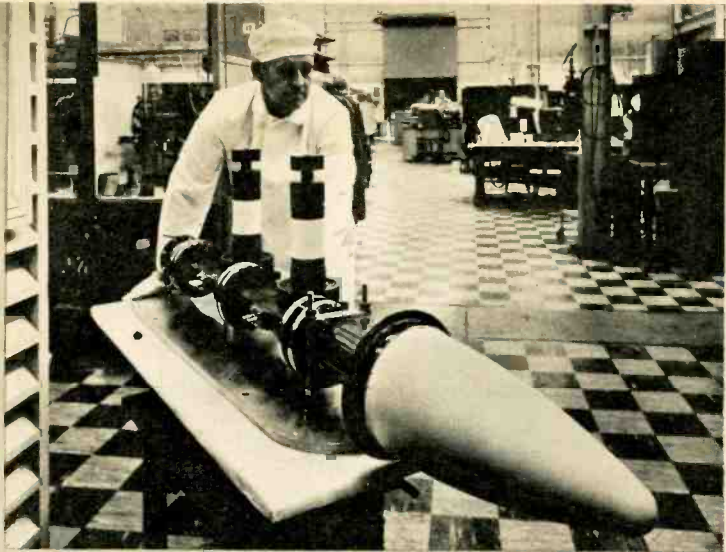
New hope for Tesla's dream lies in Raytheon's Amplitron. No paltry powerhouse, the tube can produce some 425 kw of microwave power, nearly 100 times the amount used in the model-helicopter experiments.
