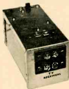
Fig. 4—Power supply is a bit crowded. The battery holder is mounted on a homebrew aluminum bracket over transformer. Terminal strip TS5 on top of cabinet is for twin-booster. TV sets are connected to the terminal strips at end of the cabinet.
