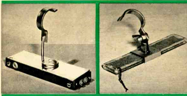
Fig. 5—Booster (left) and solar cell (right) are mounted on mast with home-brew brackets made from twin-lead clip-on standoff insulators. Watch the pressure on the solar cell or its case may crack. Apply waterproofing material or tape to booster-case seams and the wire hole on the solar cell to keep all moisture out.
