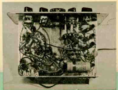
Underside of receiver is crowded. You must be careful to position leads where shown in manual or else the IF stages will break into oscillation.
