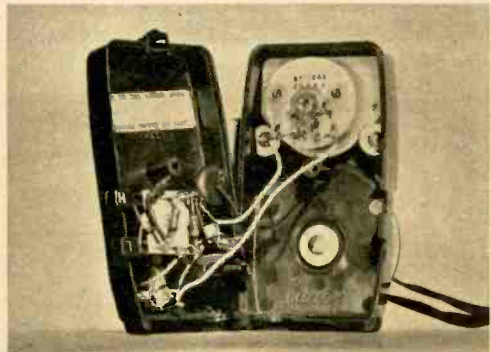
Interior of wired meter shows computer back at lower right and meter terminals at upper right.
