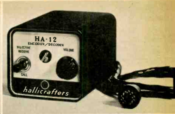
HA-12 by Hallicrafters incorporates a call light, plugs into company's CB-3A transceiver. $79.95.
