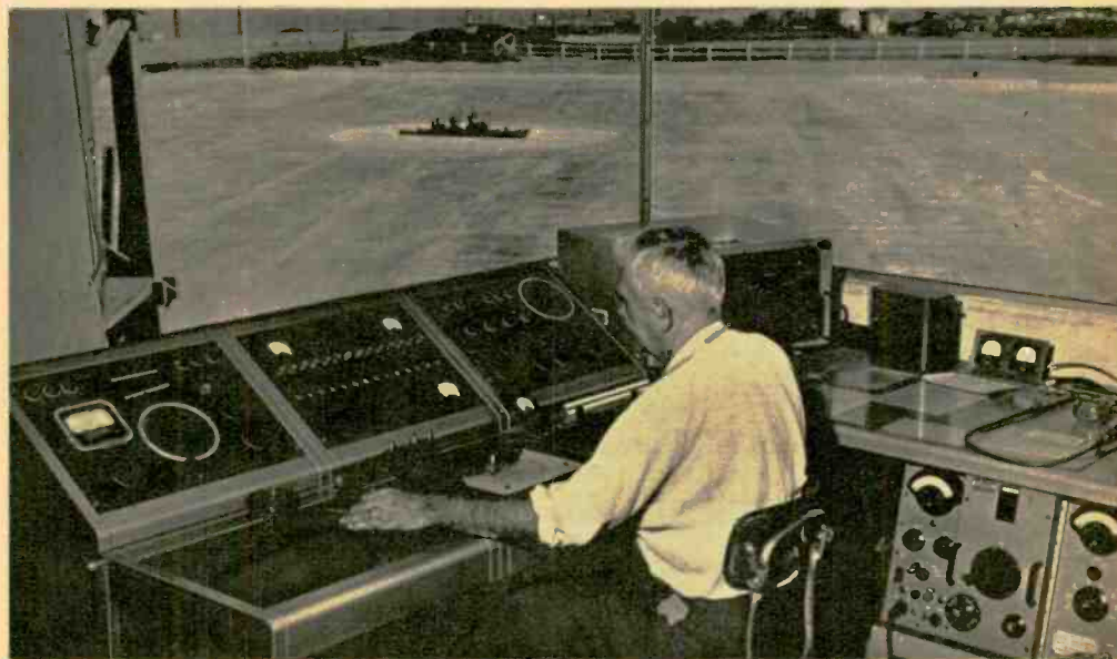
Technician Leo P. Wilbert sits at the control console of the half-pint antenna lab. Model ship in man-made ocean rests on a revolving turntable, enabling pickup patterns to be charted for most any angle.
