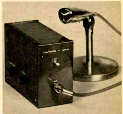
A useful accessory for hams and CBers, the Compressor-Limiter will fit in a 3x5x7-inch Minibox.
