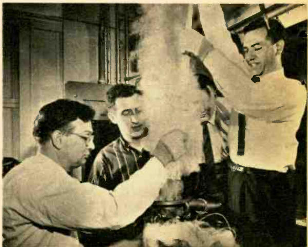
Helium rises in smoke-like fashion as super-magnet is withdrawn from super-cold, liquid-helium bath.
