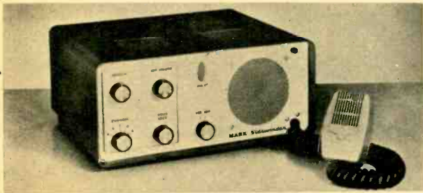
First commercial single-sideband CB rig is Mark's Sidewinder. Switch at lower center of front panel provides for selection of lower or upper sideband.
