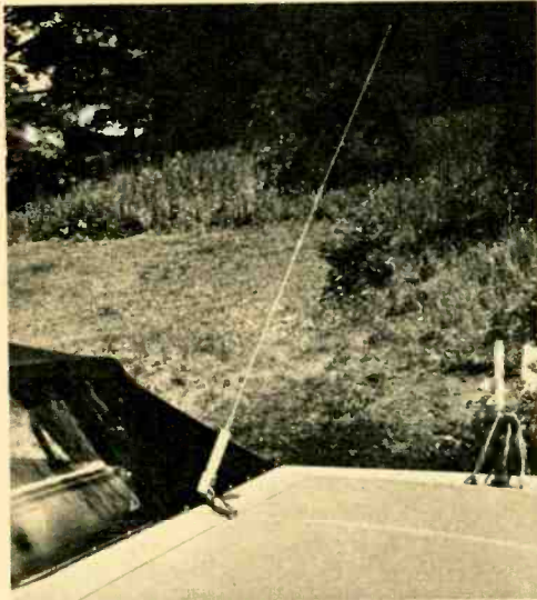
Loaded whip for rear-cowl mounting has a rakish look. It's made by Antenna Specialists.
