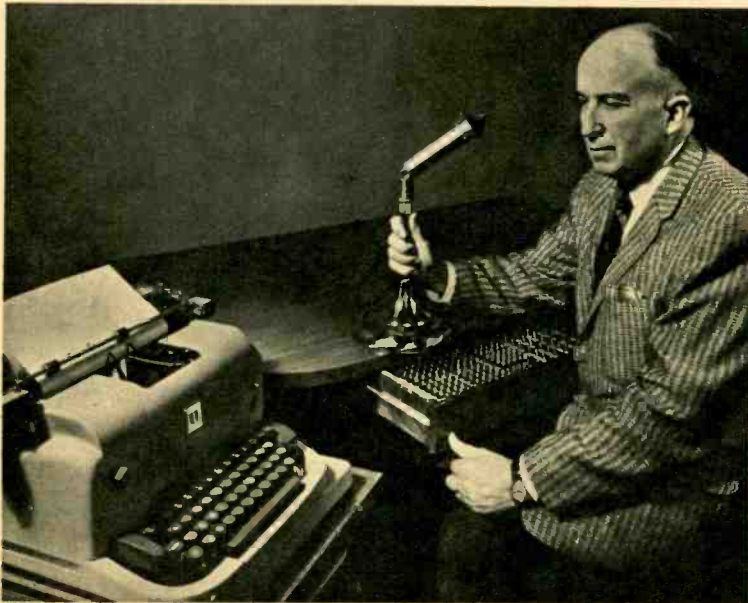
Phonetic typewriter developed by RCA's Dr. Harry F. Olson identifies words by breaking sounds into component frequency bands, then determining the duration of the sounds in each band. Though its vocabulary is limited to 100 syllables, this experimental machine is capable of typing words spoken into the microphone. System functions much like a human ear and brain in analyzing the sounds that it hears.
