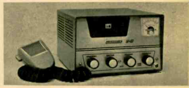
Frequency synthesis is featured in Hammarlund's CB-23 all-channel CB transceiver. Operator first dials channel range, then selects specific channel.
