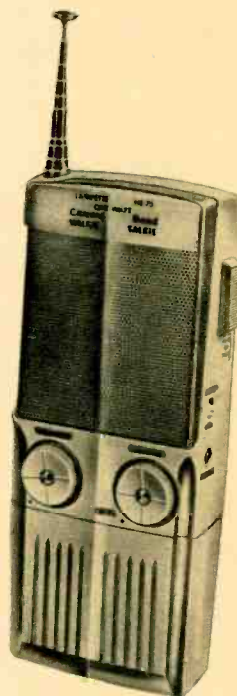
HE-75 walkie-talkie by Lafayette includes a crystal-controlled super-het receiver. Transmitter is rated at 1 watt.
