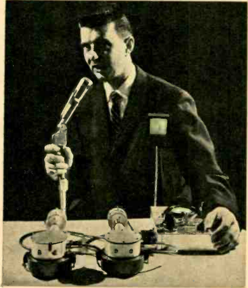
Sperry Gyroscope's Sceptron can listen to, understand and react to human commands. Mask which programs machine is interchangeable, so device can be made to recognize most any word.
