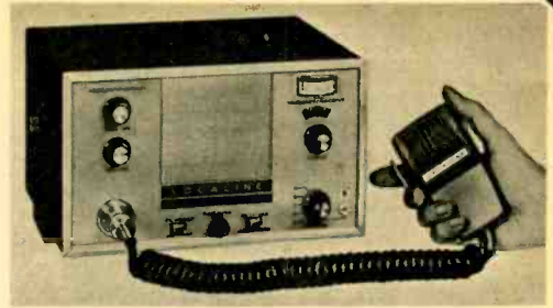
Trend toward transistors in CB equipment is typified by Vocaline's ED-276. Transistors appear in receiver circuit tubes in audio and transmit sections.
