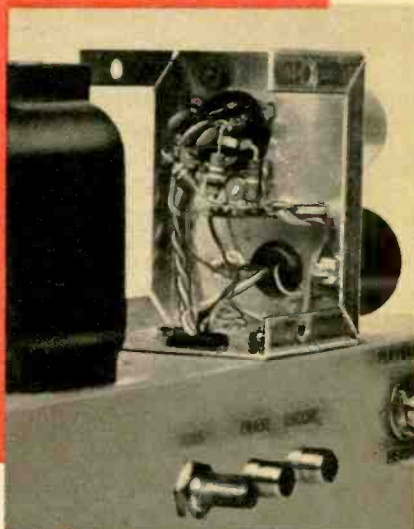
Bias oscillator subassembly is made up of separate chassis box mounted on top of main chassis. Bottom cover has been removed from subassembly in photo at right.
