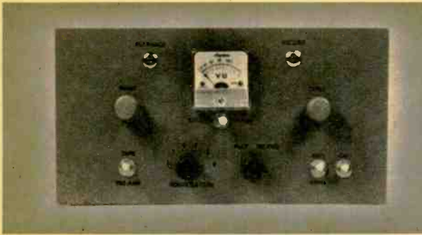
Completed tape record preamp makes an attractive addition to any hi-fi installation. Self-contained preamplifier tube feeds into record preamp for recording or into external amplifier for playback.
