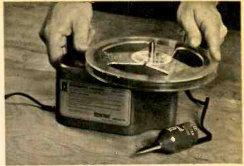
Two essential tools for tape-recorder care are the head demagnetizer (the small, pointed instrument in the foreground) and the bulk eraser (the large device holding the reel of tape in the photo). Used periodically, the head demagnetizer cancels residual magnetism on tape heads. And the bulk eraser completely removes signals from tapes, reducing head wear and leaving tapes in like-new condition.
