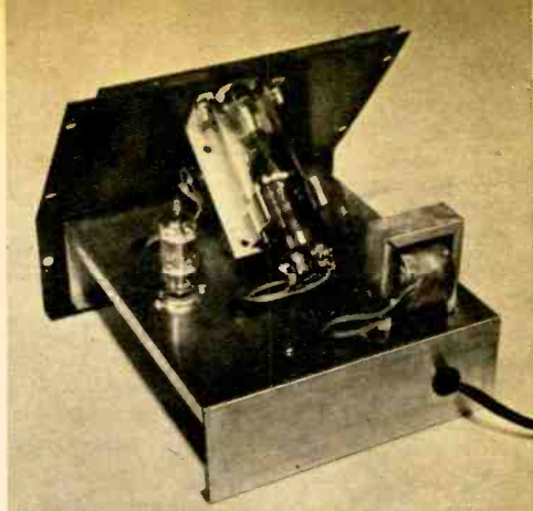
Top-chassis view. Wattmeter could be built in a smaller cabinet if portability is important.
