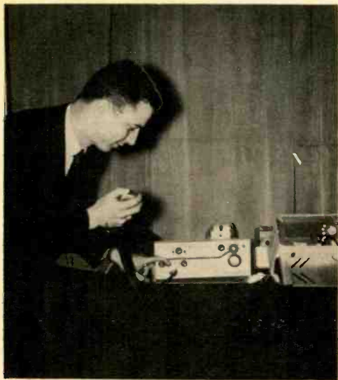
Polytronics booth had new frequency synthesis rig that gives you 23 channels on 12 crystals.
