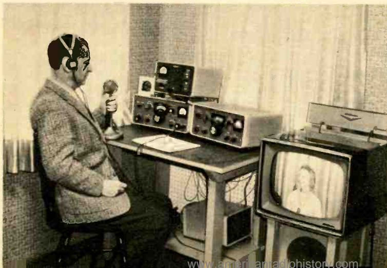
W2DJJ enjoying luxury of an expensive SSB rig that he's keeping warm while the real owner tries to pass his code test for a ticket. He uses TV set in the foreground to show absence of TVI, although his two antennas are less than 10 ft. apart. TV image was so bright even flash didn't kill it when photo was made.
