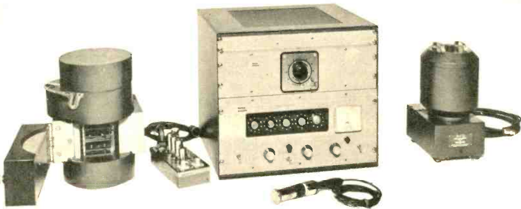
Medical isotope equipment includes Geiger counter (left), scintillation counter (right). Computer in center registers readings from either unit.
