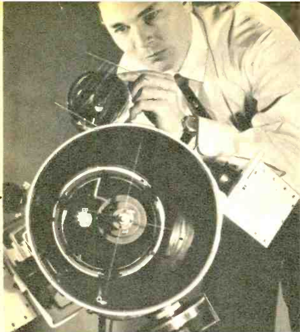
Business end of Hughes light radar shows optical maser transmitter in small tube on top of the reflecting telescope receiver. Detector, amplifier and associated circuitry are in box on instrument's side.
