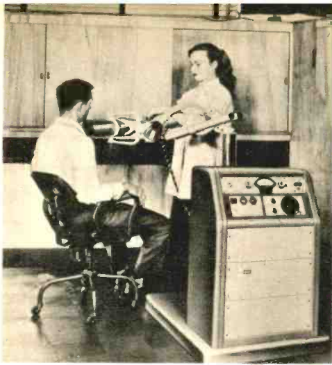
A scintillation counter to which is attached a collimator is used to measure the uptake of radioactive iodine by patient's thyroid gland.
