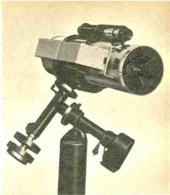
Business end of Hughes light radar shows optical maser transmitter in small tube on top of the reflecting telescope receiver. Detector, amplifier and associated circuitry are in box on instrument's side.
