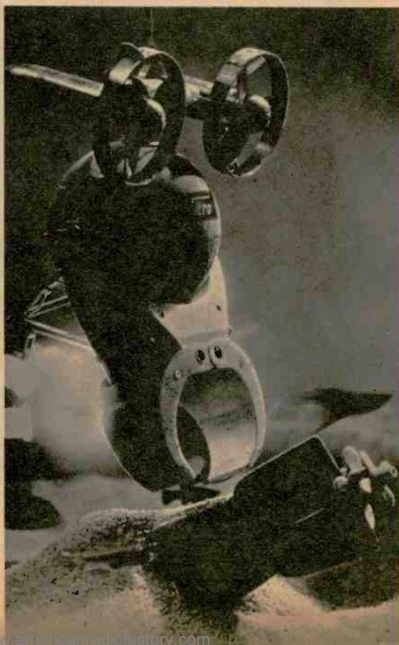
Huge claw of Solaris, a one-eyed robot built by Vitro Laboratories, can clamp onto an object on the ocean floor and then lift as much as 7,500 lbs. to the surface. It is controlled from aboard ship by the operator above. Unit includes TV camera and lights at rear, two props for maneuvering, mechanical power unit in sphere. It operates at end of two cables, can go to 2,000 ft.
