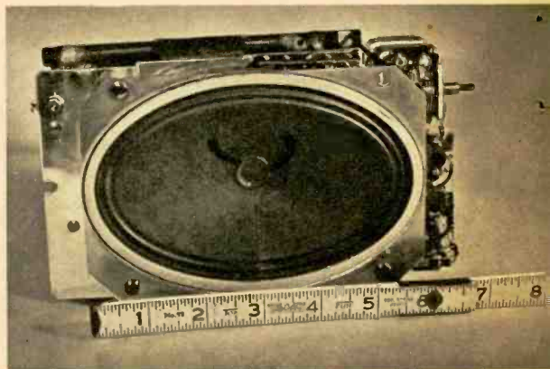
Sizable speaker provides excellent volume and tone. Case dimensions are 8½" x 4½" x 2¼".
