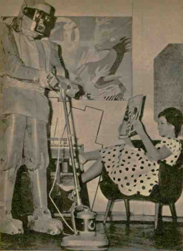
Mechanical men out of fiction and the amateur workshops tend to look and act a little like the real thing, although human form and actions are illogical for machines. This is MM7, built by a Viennese engineer. It can pour a drink into a fragile glass without breaking it, also startles guests by polishing floors (left). Elaborate control panel runs the 6-foot robot.
