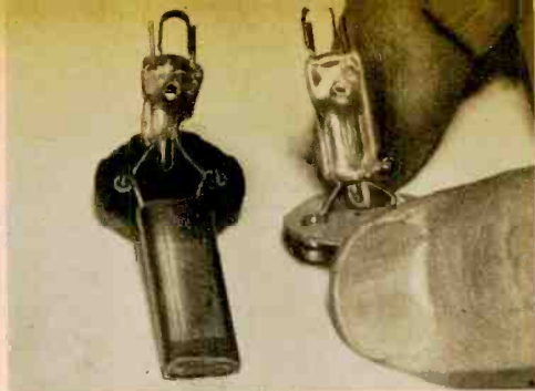
Starter used for SW1 is separated from base, soldered to flea clips, and centered in R1.
