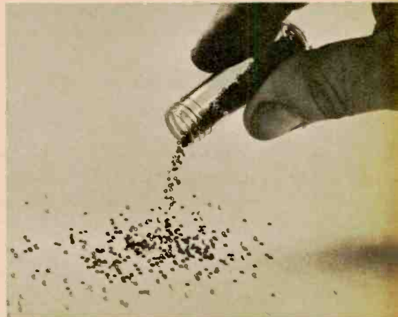
Each of these ferrite doughnuts represents a single memory core for a modern computer.
