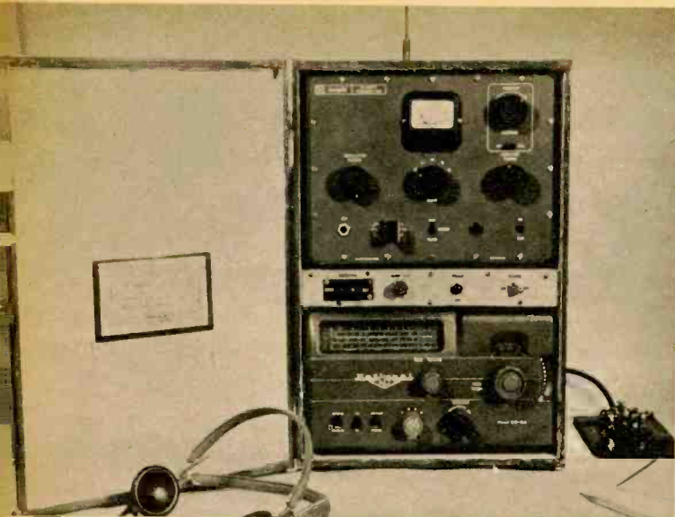
Control panel fits into space between Knight-Kit 50-watt CW transmitter and the National SW-54 receiver on the bottom. Note key and phones.
