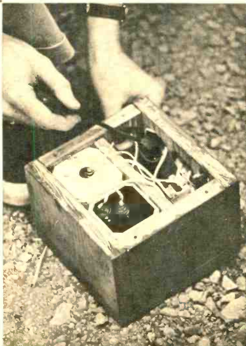
The only "electronics" at the Advanced shoot was this battery box, left, with mercury switch (tripped by thread tied to rocket) to actuate a camera. Right, a successful launching, the exception rather than rule at shoot.
