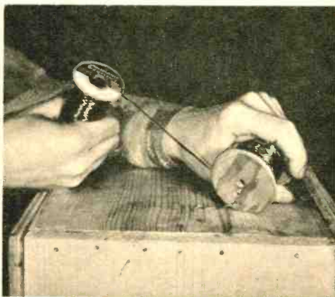
Wind the coil for the crossover network fairly tight. Make certain that you fill up the coil form evenly with 400 turns of wire.
