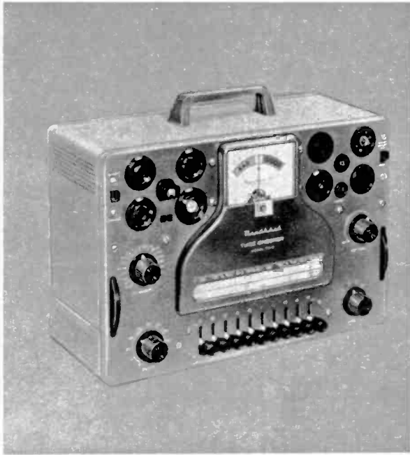
Fig. 10. Another kit emission tester. Data for checking is on roll chart, above switches.
