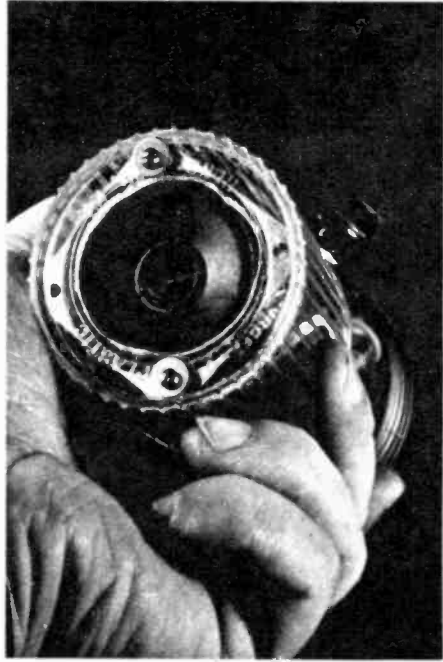
Hole in closed end of glass is cut for speaker, secured in place by two screws.
