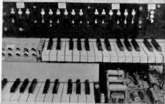
Top panel holds voicing and stop switches. Last switch on right is set low, medium or high volume; adjusts speaker level to center of dynamic range.
