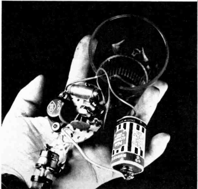
Basic components removed from glass include electronic sub-assembly, battery, and volume control.
