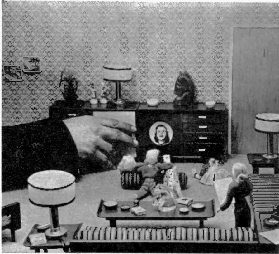
Television set in miniature home actually works. Although screen is tiny, the other parts of the set extend for about a foot beyond back of display.
