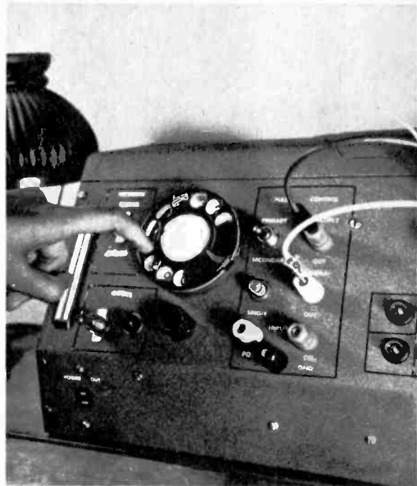
The computer is fed by the telephone dial. To add 4 + 4 dial the number 4 twice in succession.
