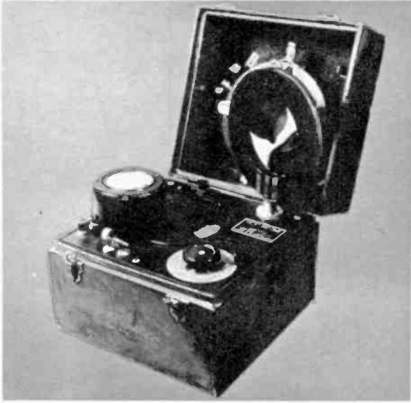
Here is famed Kolster Decremeter, used by pioneer Radio Inspectors to check emissions of spark transmitters. Pickup loop is at right, RF galvanometer at left behind crystal detector.
