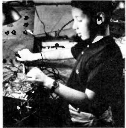
Here audio signal is fed through a hi-fi amplifier and observed on oscilloscope.
