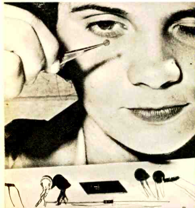
Small silicon slice does everything that transistorized oscillator (parts shown) will do. Westinghouse photo
