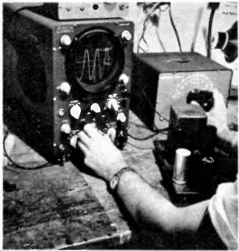
Here audio signal is fed through a hi-fi amplifier and observed on oscilloscope.
