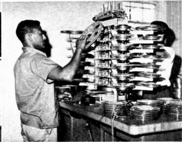
. . . very fast hands remove the completed tapes. Tape heads can be changed from monophonic to two- and four-track stereo easily.
