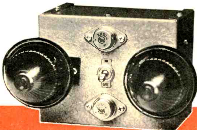
Lamps and two power transistors are on outside of case. Wiring guide is below.
