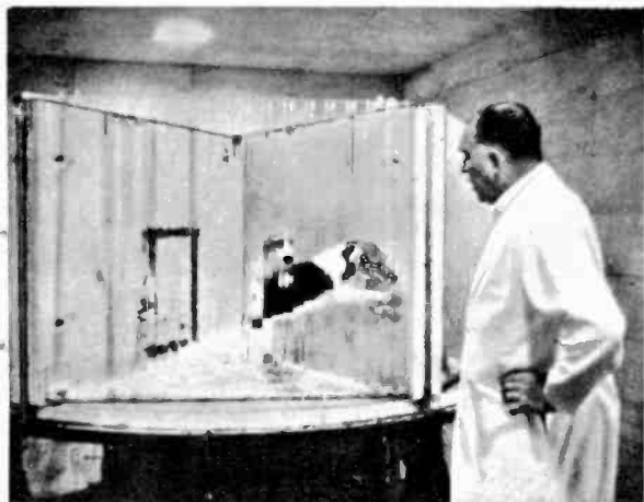
At left, Dr. William Deichmann pauses to look over rotating table partitioned with Plexiglas. Animals in each section are exposed to radar.
