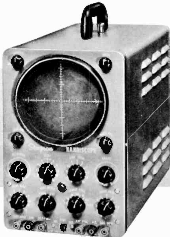
Fig. 4. A 1 volt peak-to-peak calibrating voltage is supplied by a terminal at lower left. It is the third post from the edge.
