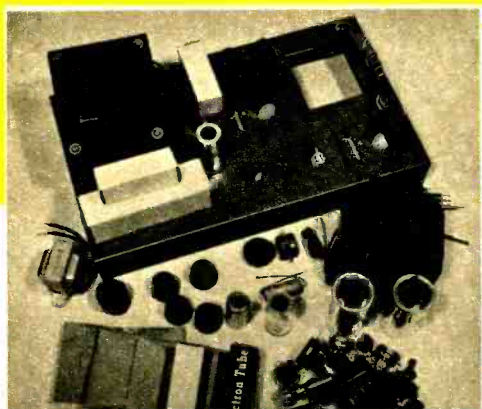
Layout of parts after kit is unpacked. Large chassis is made of steel plated with copper.
