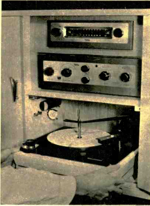
A Glaser-Steers changer is installed in left section. Note 45 RPM spindle, adapter and spare fuse on side wall. Above is EICO stereo amplifier and FM tuner mounted in upper panel. Bar is in right section, shown rotated to about half-open position revealing shelves in rear.
