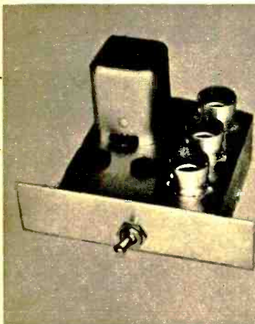
Shield-type tube sockets are used on small chassis. Can see oscillator transformer T.
