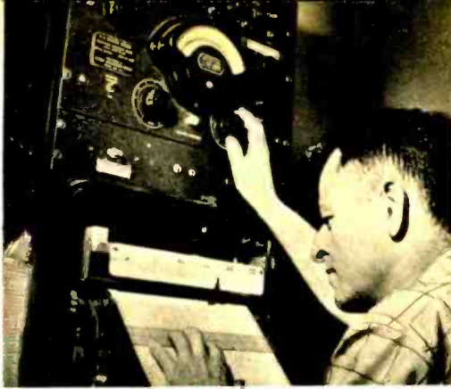
Operator tunes receiver and checks graph read-out of humidity, air pressure and temperature as relayed via UHF radio.
