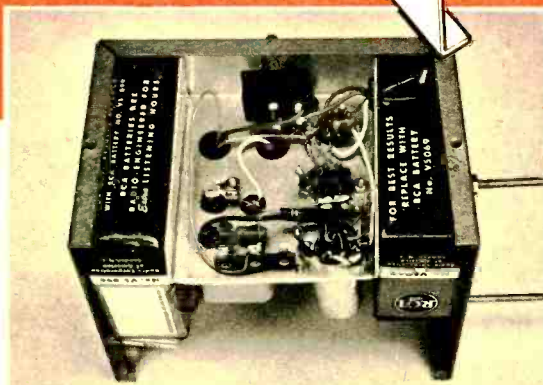
In wiring guide above, small chassis has been raised for clarity. J1 is insulated from case—it carries 90 volts from B1.
