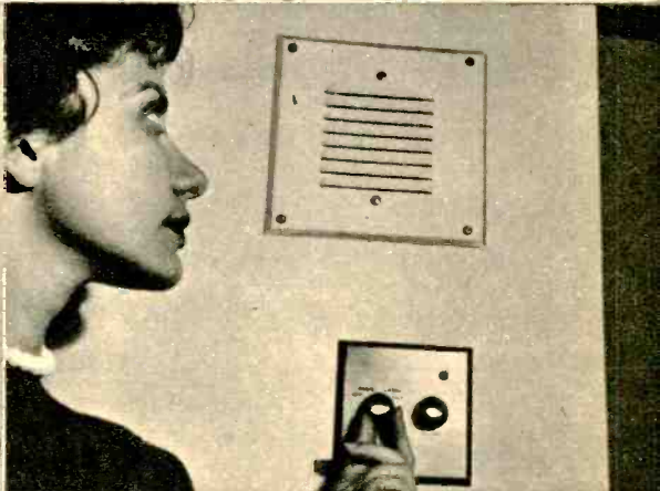
Speaker is bolted to grille, wires soldered. Slack wire will permit removal for servicing.
