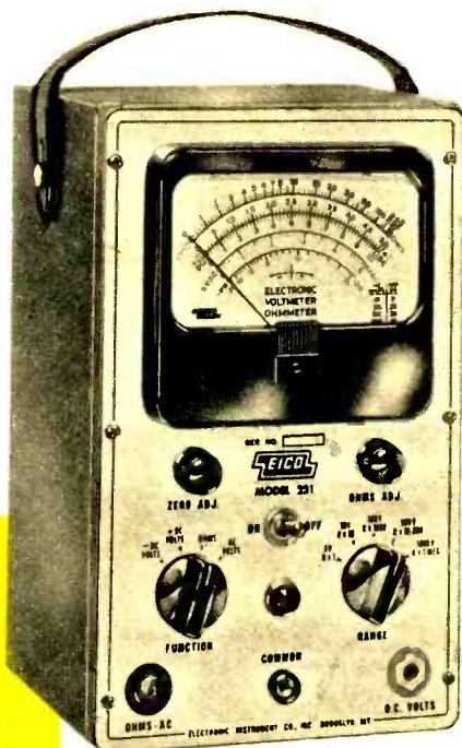
Fig. 1. This VTVM is set up to read resistance—RX10,000.
