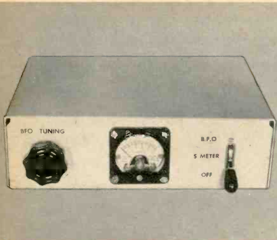
Front panel of the unit. BFO tuning changes pitch of code signal. S-meter is at center.
