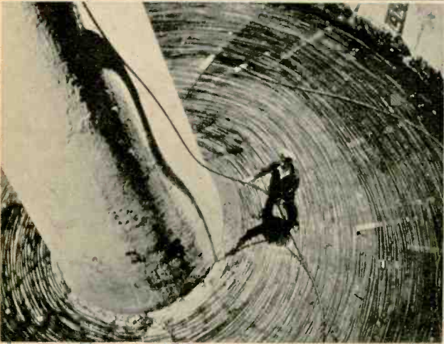
Cable aboard the Monarch is kept in one of four huge cable tanks such as one at left. Operated by American Telephone and Telegraph Co., she can carry about 2,000 miles of cable at one time. The present submarine cables cost over $42-million.
