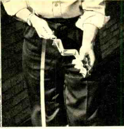
Brackets for chimney mount come with two metal straps usually 10 or 12 feet long.
