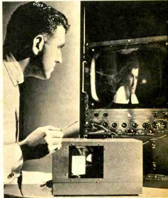
This Avion CODES gear is slated for IR satellite detection. Note cigarette "burn" on scope.
