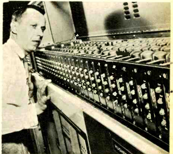
Engineer at Hughes Aircraft glances down the one bank of circuitry through which all information to milling and boring machines is fed before it is converted into pneumatic actions.
