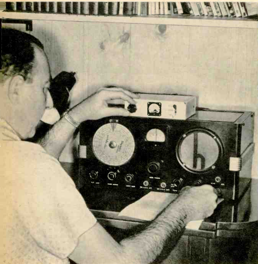
Unit may sit atop receiver. S-meter needle rises and falls as stations are tuned. Author is adjusting BFO for pleasing tone.
