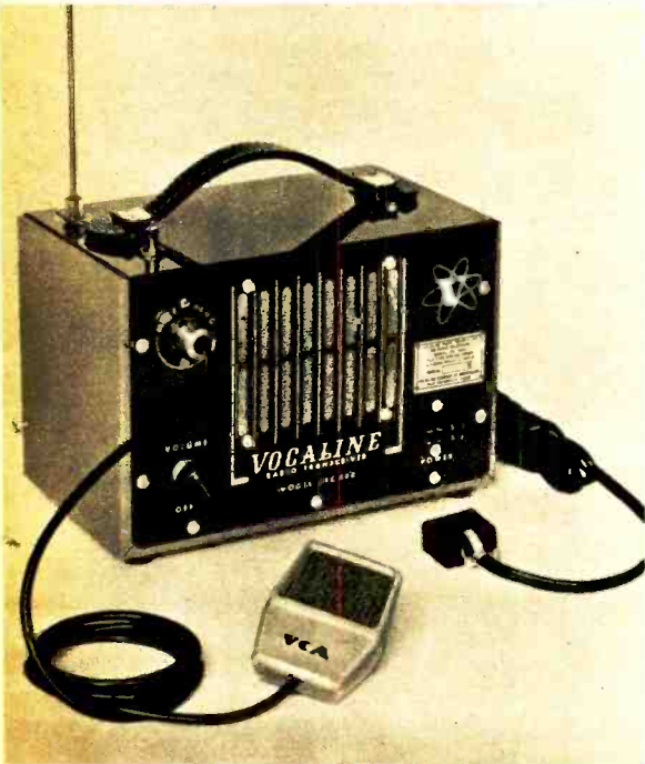
This Vocaline transceiver is for class B only at 465 mc but, class D gear may be forthcoming.
