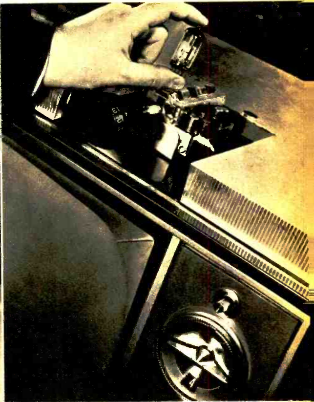
Using only a fraction of the plate power of conventional television tuners, this set gave improved reception with a "nuvistorized" tuner. Hand holds "large" miniature tubes.
