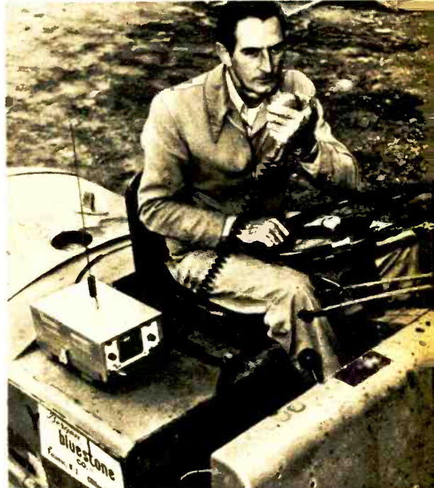
Class D Citizens radio may also be used for business as is this Kaar Engineering Corp. unit.
