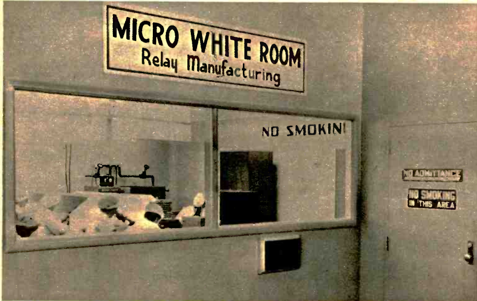
Final assembly room of G-E miniature relay plant in Waynesboro, Va., is typical of anti-septic precautions taken in miniaturization. Sealed off from rest of building, assemblers work over microscopes in room where the temperature and humidity of dustless air is very rigidly controlled. Right, inspector electronically tests friction of miniature ball bearing.
