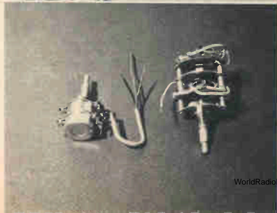
The balance control, far left, and function selector, right, are both dual controls, wired before being bolted to panel.
