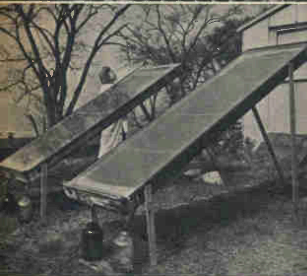
Silicon cells, 144 in all, are linked together to charge batteries rated from 6 to 48 volts.
