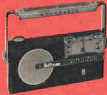
Now on market is this transistorized portable radio. Solar cells are embedded in the handle.
