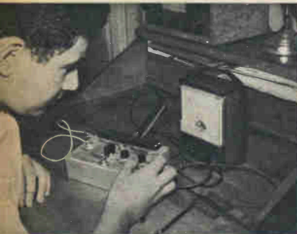
With a meter added, the unit is able to check the operation of its own or other transistors.
