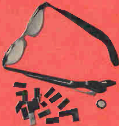
Eyeglass hearing aid by Zenith recharges miniature battery from silicon cells on temple bar.
