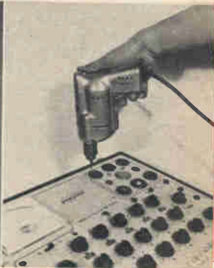
Pilot holes are drilled in carrying case to receive the panel wood screws.
