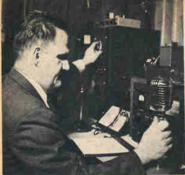
Gunderson fires up rig by a unique telephone dialing system of his own design. It controls power, tuning, and band of homebrew transmitter.
