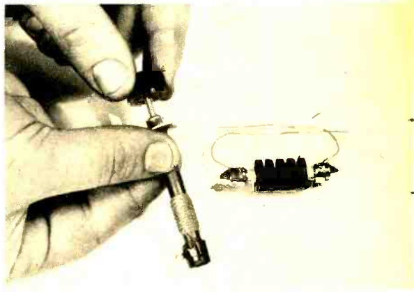
A variable inductor being tuned, and a fixed RF choke used for blocking high frequencies.
