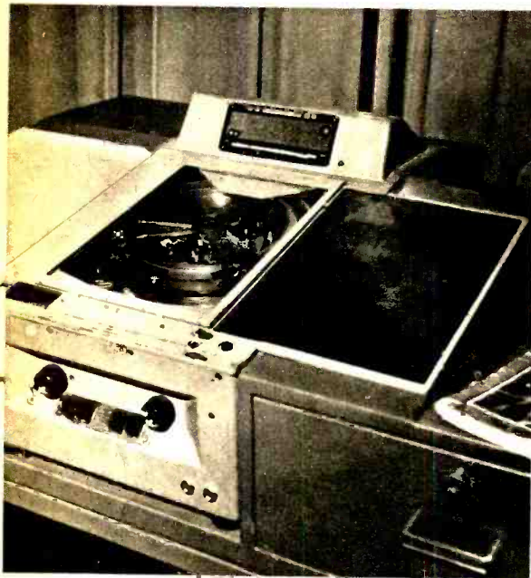
This model has Synchrosheet removed to reveal turntable containing recording heads.
