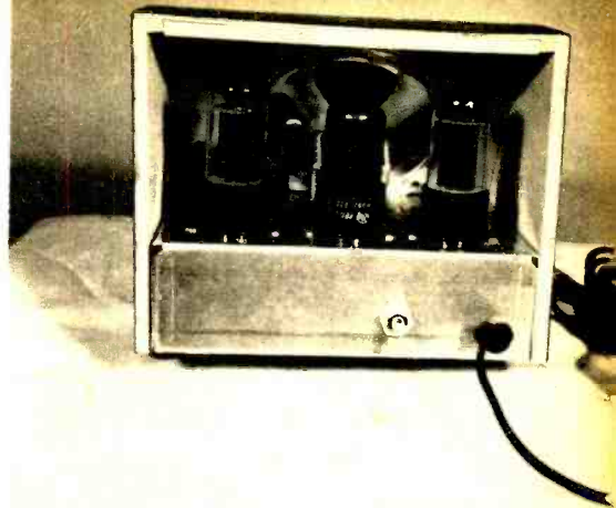
A simple wood cabinet encloses the unit. It is anchored to speaker frame and chassis.
