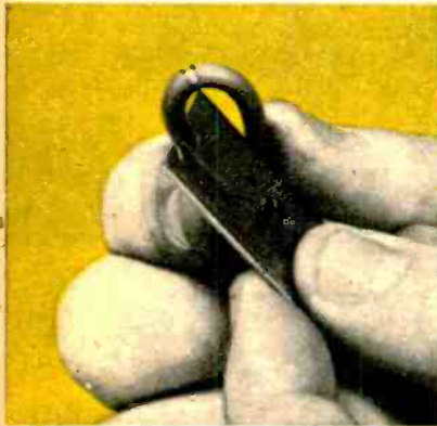
4A. Strip shielded cable this way. First remove plastic jacket carefully with razor.
