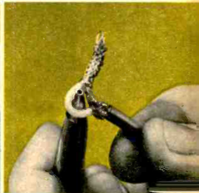
4C. Form a loop with the inner conductor and pull it out of the hole in braid.
