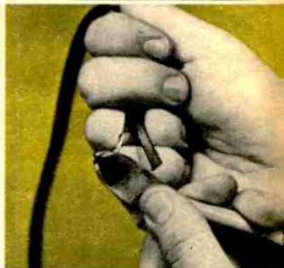
5C. Pinch edge of plastic without cutting through and twist off. Bare wire remains.
