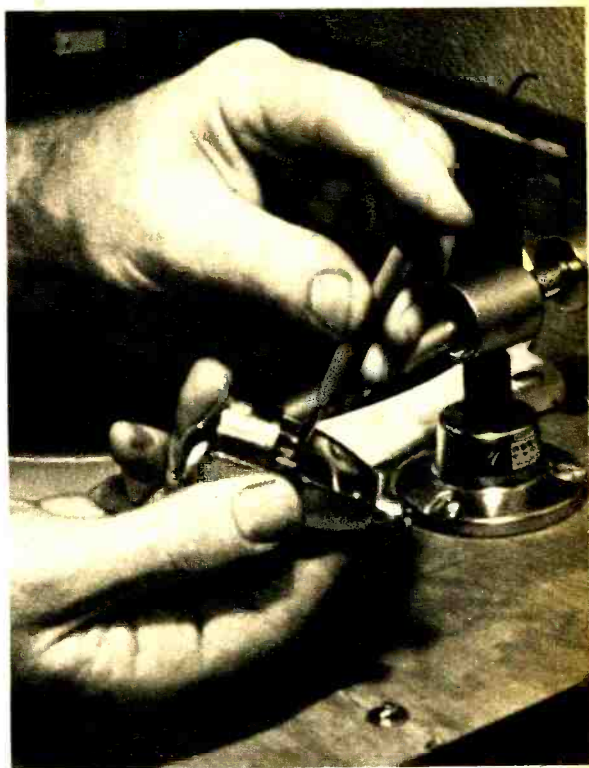
The cartridge must be mounted squarely in the tone arm, or shell, as in the type above.
