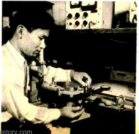
Semiconductor diode (in right hand) is mounted in unit which tests amplifying properties. Bell Labs
