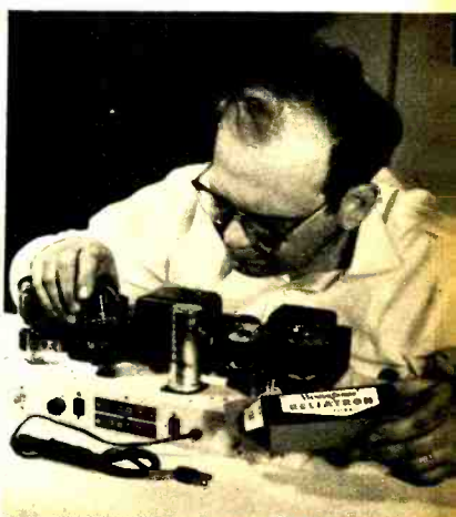
If all filaments light, then the rectifier is plugged in.
