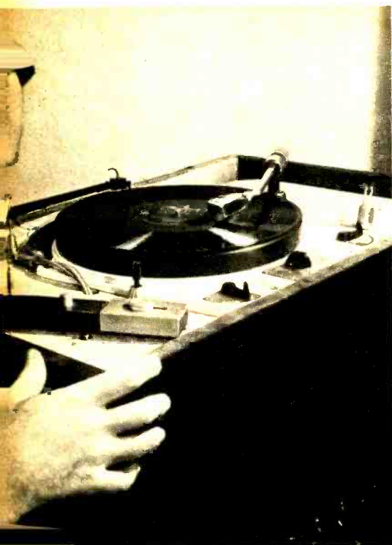
Sight the cartridge by viewing its reflection on the record. Any unevenness will show up.
