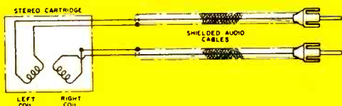
4-terminal pickup keeps internal and external grounds isolated until they reach preamp(s).
