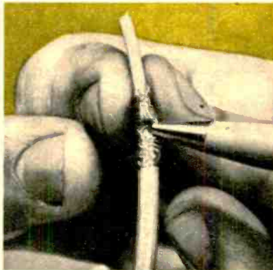
4B. Push back the braid until it bulges. Gently work an opening in it as shown.
