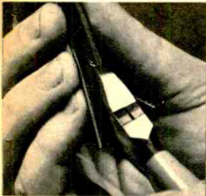
5A. Strip TV twinlead with cutters. First cut an inch up the center of the plastic.
