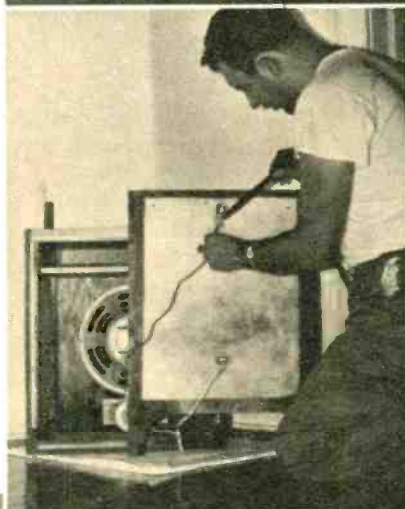
Then speakers are mounted on front panel and the L-pad is wired.
