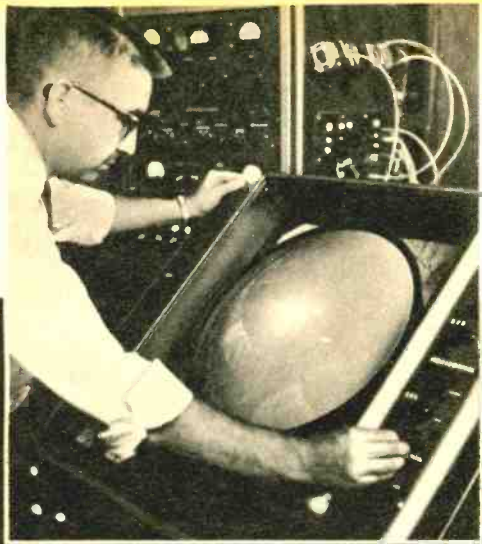
Charactron air survey display gives instant and steady target identification, altitude and speed. Set of 9 characters, "written" electronically on screen, corresponds to an airplane's position as determined by radar.
