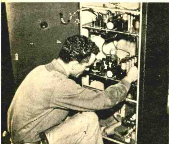
Accuracy of color scanners on presses are monitored by this bank of electronic gear.
