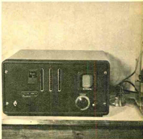
Apparatus does blood counts electronically in 15 seconds by counting 50,000 cells per sec.
