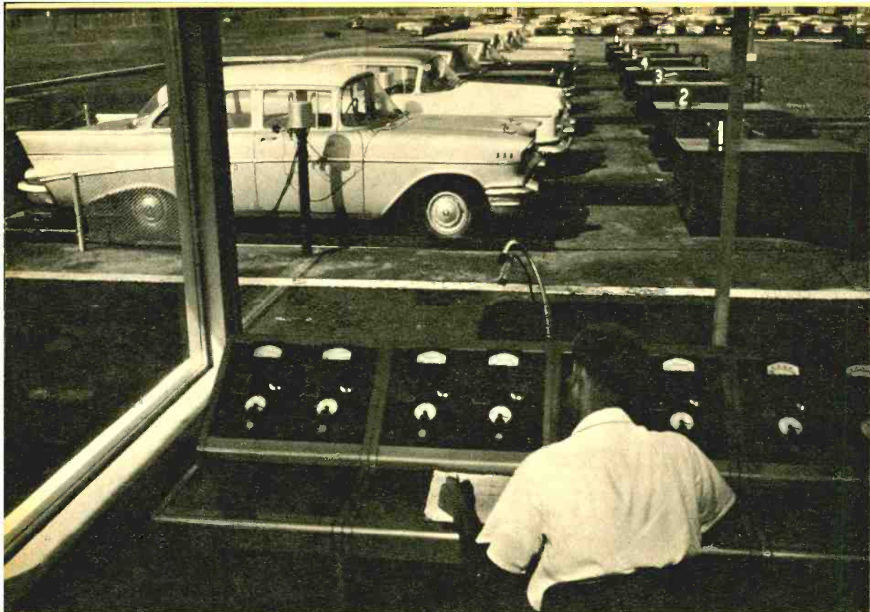
View from control room shows control consoles and eight test autos being put through paces on treadmill, each car duplicating a recorded road trip.
