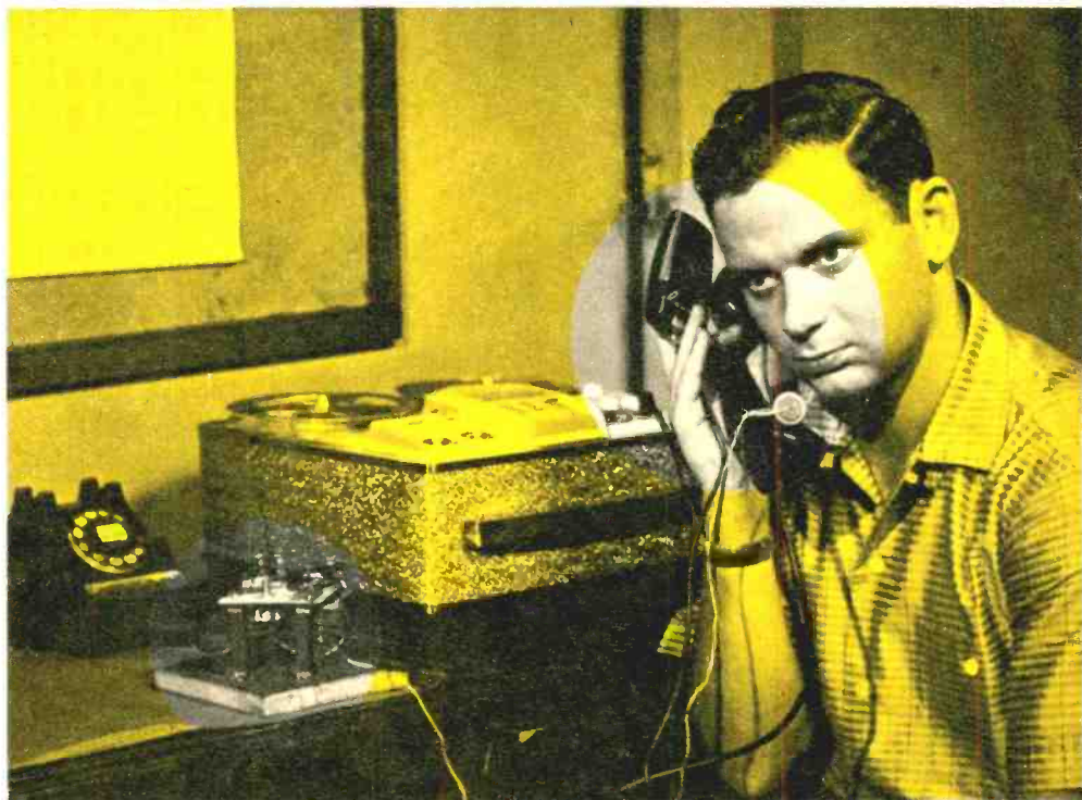
The Beeper, seen at lower left, feeds its signal to the earphone mounted on telephone mouthpiece. Person at other end of the line hears the tone.
