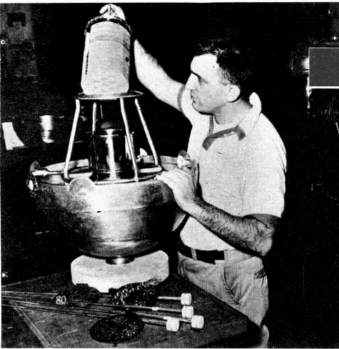
The electronic circuits responsible for the gathering and coding of space information obtained by the Vanguard satellite are contained in the cylindrical unit shown being lowered into the satellite. This unit consists of printed circuits of the type on the table. Antenna elements are also shown in the foreground on the table.
