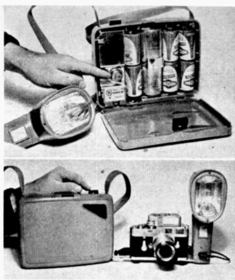
Top, inside of Mecablitz 100 flash unit. Finger indicates transistor, oscillator is under shield. The complete unit as shown above is book size, note position of convenient on-off switch.
