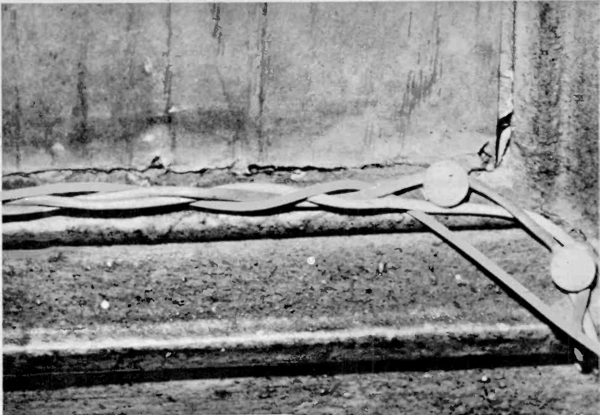
Core and semifinished pickup coil covered with Scotch tape; note reinforced leads.
