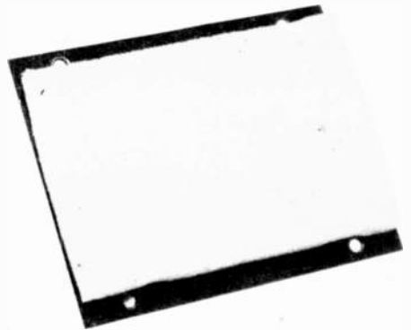
Glue a piece of foam rubber or plastic to bottom of transmitter to ease vibration.
