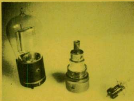
Fig. 1 Trend to high-frequency tube design. Left to right: 201A, lighthouse tube, acorn tube.
