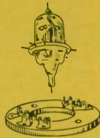
Fig. 2 Basing and socket arrangement for the acorn tube.
