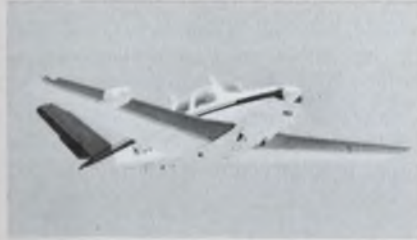
Radome on wing's leading edge contains weather radar system.
