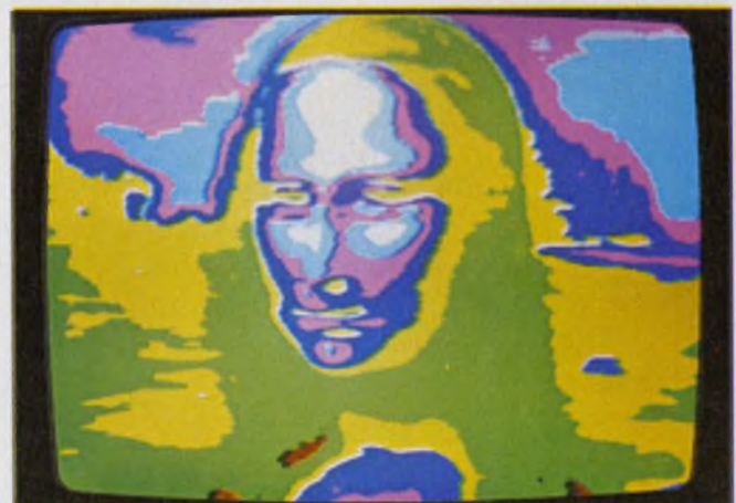
The Mona Lisa in eight grey levels and in eight-level pseudocolor (colors arbitrarily assigned to grey levels) demonstrate the capabilities of raster-scan graphics. The color image is produced on a standard color monitor.
