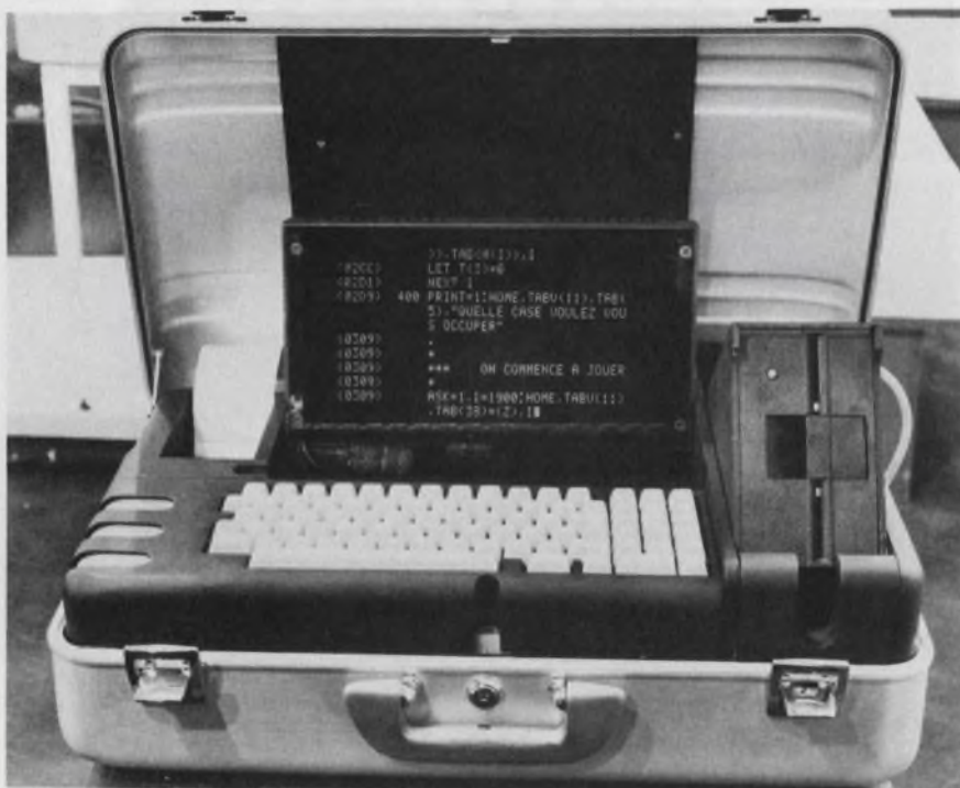
5. This well-stacked \mu C in a suitcase contains a plasma display, floppy drive and printer. It comes from R2E (France), and obviously speaks Le Basic.
