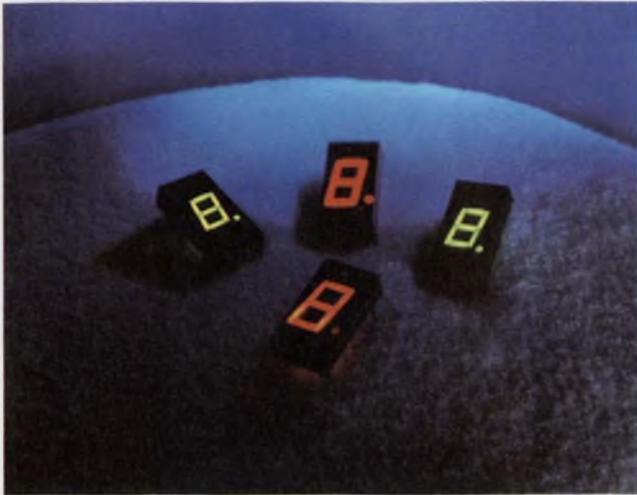
Four colors of seven-segment LED readouts —red, orange, yellow and green—are now available. The 0.3-in. multi-color devices by Monsanto are mounted in arrays with 0.4-in., center-to-center spacing.
