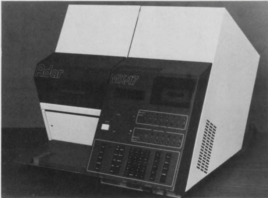
By comparing against a known-good device, the Adar MX-17 can tell whether a test device's responses to a set of stimulus signals are right or wrong.
