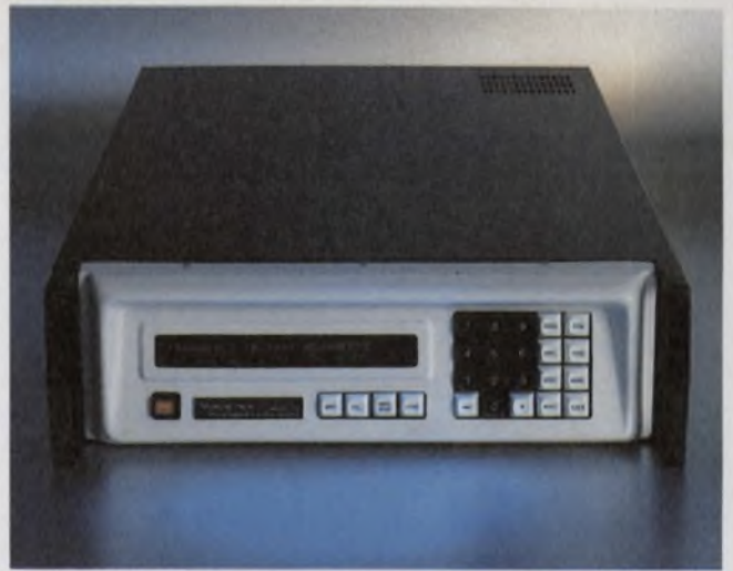
An accurate, multiple-waveform generator, Wavetek's 172 synthesized-function generator is a departure from the usual sig gen. Nine different waveforms can be generated over a frequency range of 0.0001 Hz to 13 MHz.
