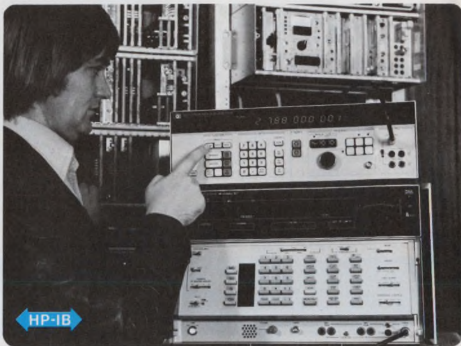
New microprocessor-based frequency synthesizer is used in applications wherever a high resolution, precision amplitude test signal is needed.
