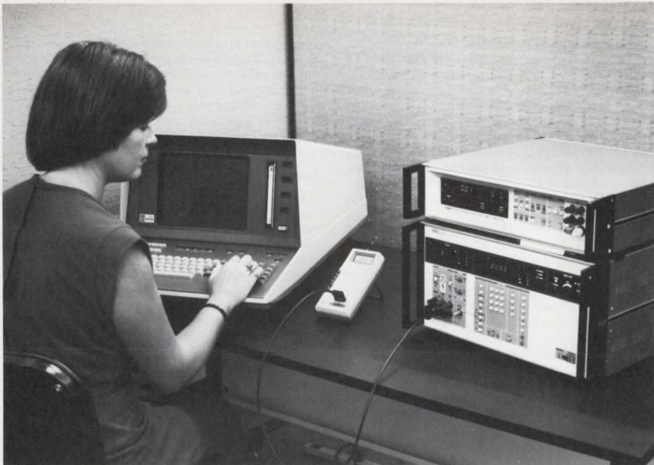
The bus puts it all together: A Fluke 5100A calibrator provides signals and an 8500A DVM makes measurements
