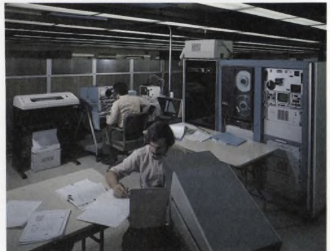
There's so much testing power built into Tektronix's S-3260 that it can test complete boards as well as ICs. All that's needed is an additional test fixture.
