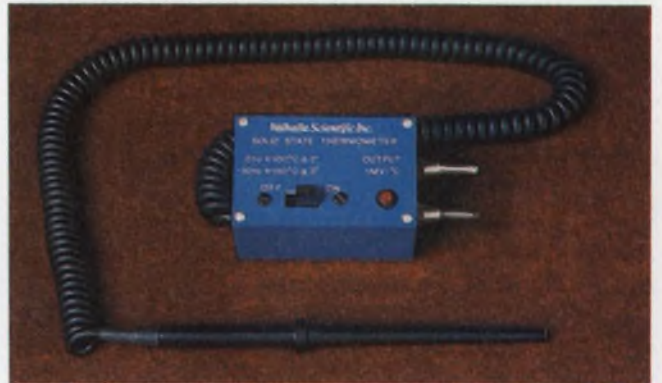
This temperature probe with a solid-state-junction thermal sensor generates an EMF of 1 mV/°C. It can be used with the Valhalla Model 4440 digital multimeter or any other DMM with a 200-mV full-scale range and autopolarity for indicating negative temperature. It can measure from -50 to 150 C.
