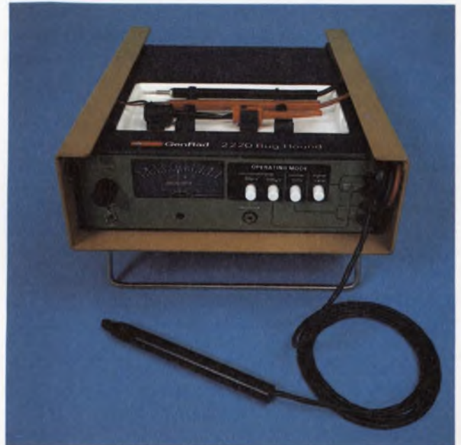
GenRad's current-tracing 2220 Bug Hound isolates faults on known-bad cards. The probe's LEDs and audible alarms pinpoint shorts, opens, bad ICs, and other troubles.
