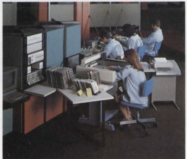
Teradyne's L125 Circuit Diagnostic System has two major configurations —one for digital boards, one for mixed analog-digital boards. By following instructions from the CRT, the operator works with the system's guided probe.
