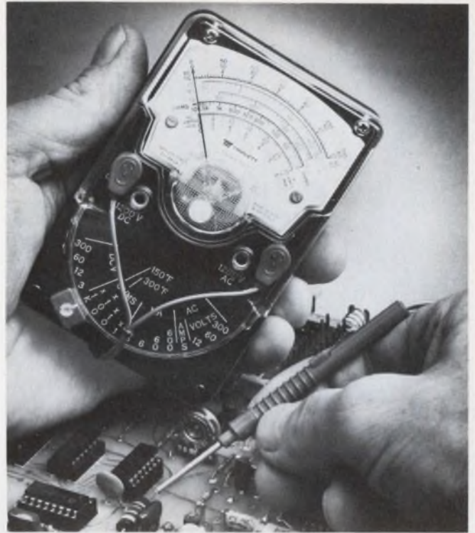
This low-cost volt-ohmmeter has two ranges for measuring temperature. The temperature probe in this Triplet instrument Model 100-T is a thermistor that measures from 50 to 300 F.
