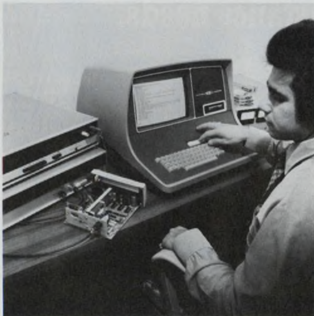
Basic-language programming and the standard bus simplify assembling test systems like this one with a Systron-Donner controller, DMM, counter, and power supply.
