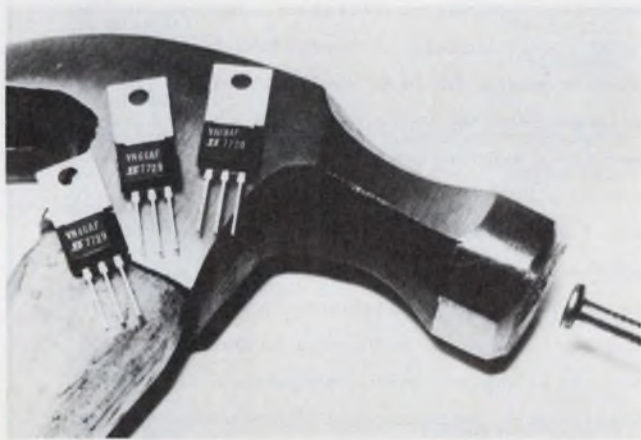
Power FETs promise to give bipolars and Darlington's stiff competition. While many companies are still working on them, Siliconix has recently announced a new series of VMOS power FETs packaged in low-cost TO-202 plastic.
