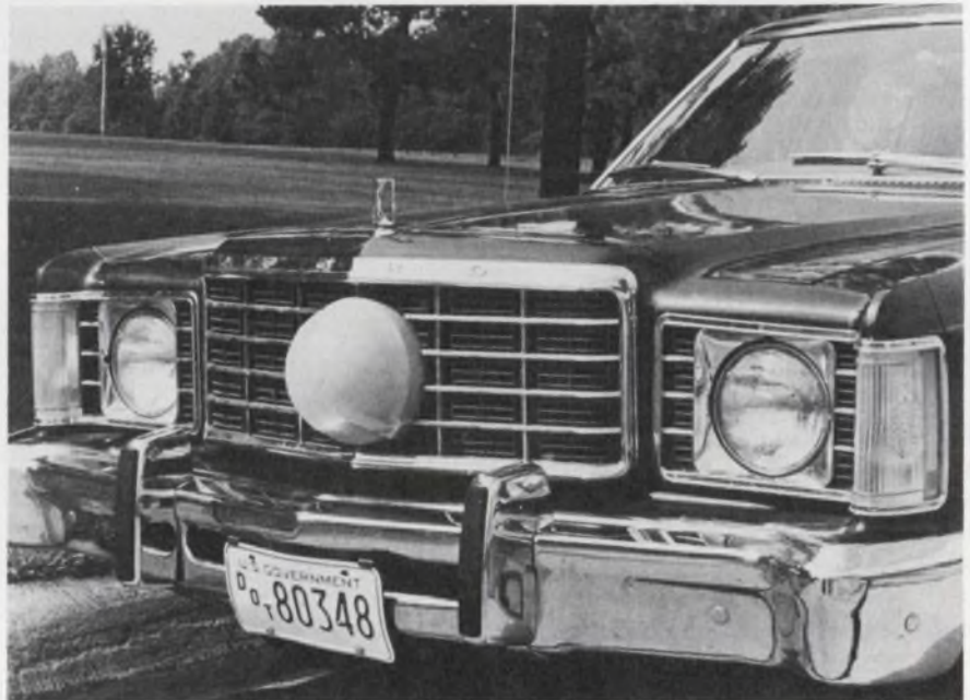
This radome for an experimental radar braking system protects radar elements from the weather. Small antenna beam width and range gating minimize false alarms that have plagued similar systems.
