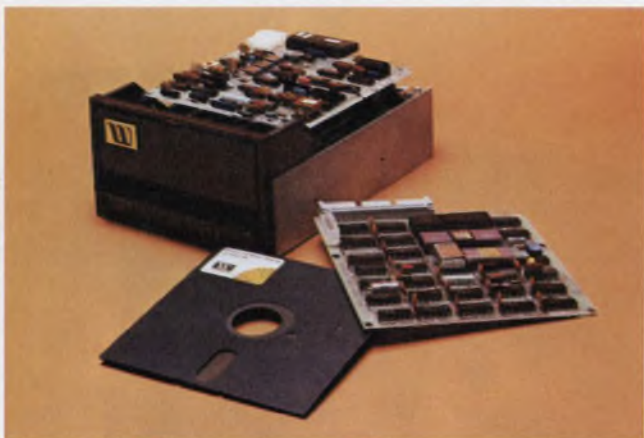
Dual-index and file-protect sensors permit recording of data on both sides of a microdiskette on the Wangco Model 82 Micro-Floppy. Up to four units can be daisy-chained on a single bus.
