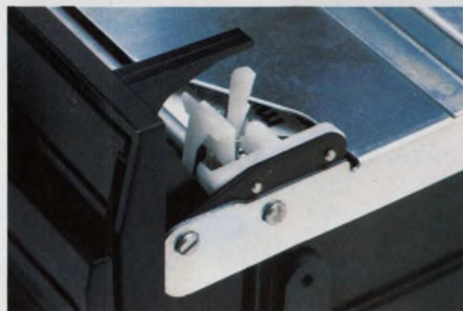
To reduce the usual disc-damage problems, Memorex 550/552 drives use a "balanced-velocity" clamping design (top) that cuts slippage during diskette engagement, and a door-controlled latch/eject mechanism (bottom) that pops media in and out and is interlocked to prevent the door from closing on a diskette that's not fully in.
