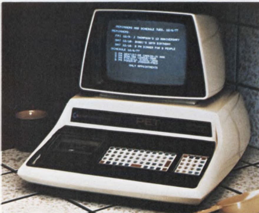
The PET computer is a complete home data-processing system that features BASIC language, a CRT display, cassette-tape mass storage and a low price tag. It costs only $595 with 4 k of RAM and 14 k of ROM.
