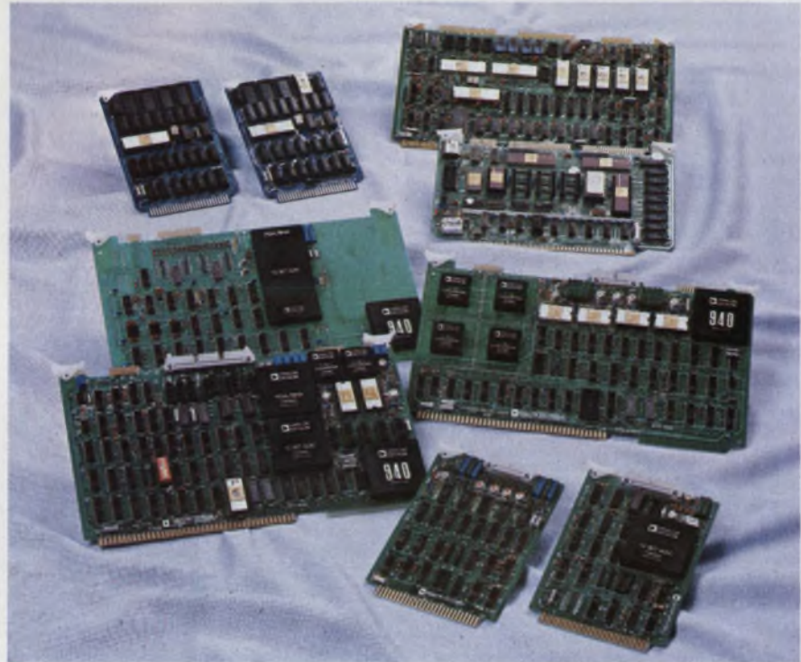
Microcomputer boards from Pro-Log, Intel and Motorola (top of picture) are seen here with compatible analog subsystem boards from Analog Devices.
