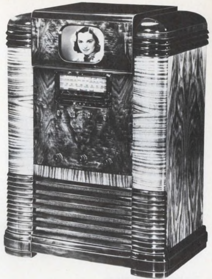
1939—Compare this set with a modern receiver. It's RCA Victor's Model TRK-9, a 9-in. model that boasted 12 vacuum tubes and included a three-band, all-wave radio chassis. It cost $450 in 1939.
