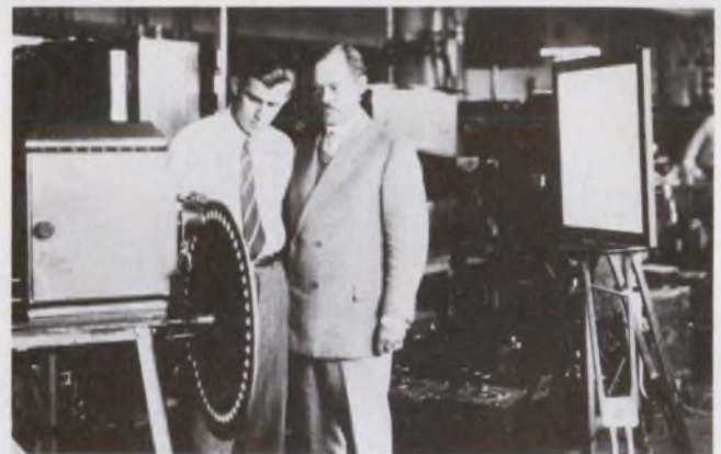
1927—Mechanical television , using Nipkow's spinning disc, dominated the early days of TV, starting about 1884. Dr. E.F.W. Alexanderson (right), the brilliant General Electric scientist, was an early pioneer.
