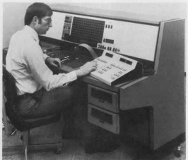
Four processors running in parallel allow the user of the Fluke Trendar 3040A to test microprocessors at clock rates up to 10 MHz. Stored sequences run at 1.5 MHz, and automatic sequences operate at 5-million patterns per second.
