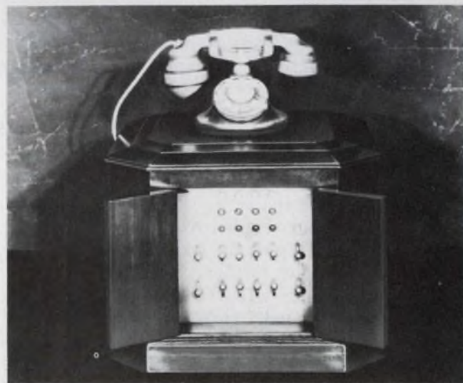
1927—The First PBX from Bell Labs featured a cordless "turret" and factory-wired switch gear to reduce installation costs. First installed in the residence of Edsel Ford, it had a prosperous 1920's look, antique walnut finish and oxidized silver panel and handset.
