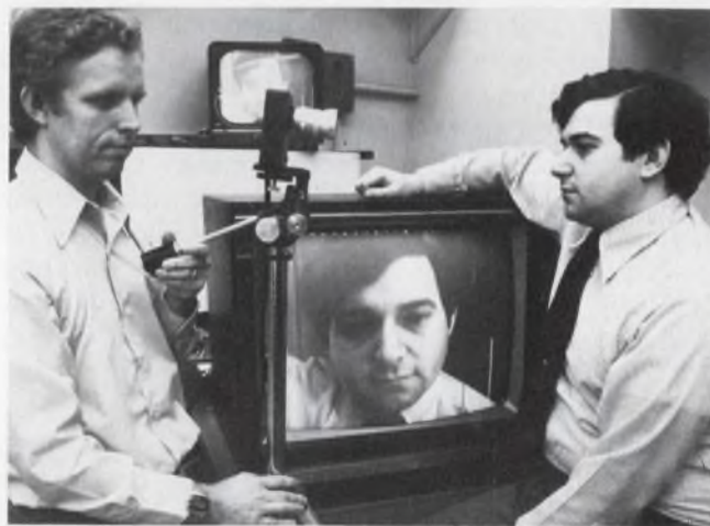
1977—Cameras without tubes shrink to inconsequential dimensions, as charge-coupled devices and other solid-state, self-scanning imaging devices begin to take over.
