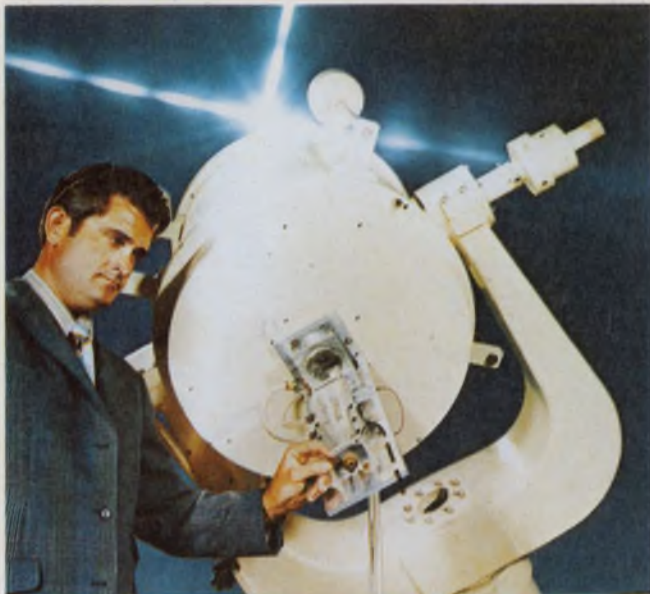
1975—A sun-powered laser was developed by GTE Sylvanica for the Air Force to test the feasibility of passing information between earth-orbiting satellites up to 43,000 miles apart.
