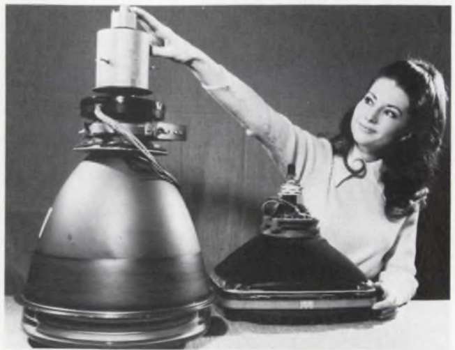
1954—Black-and-white began to give way to color in the early 1950s with the invention of the shadow-mask picture tube (left). At right is RCA's modern "precision in-line" television tube.
