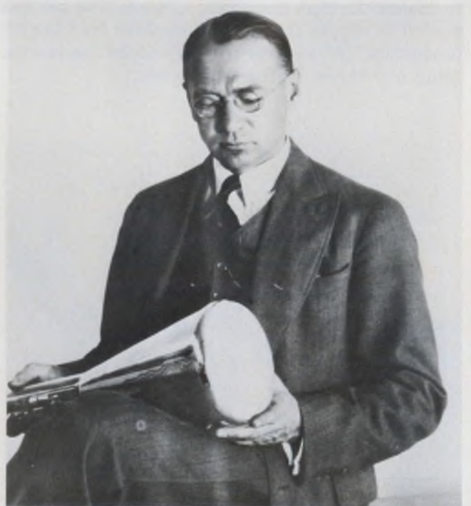
Early kinescope —or television picture tube—held by Zworykin was the second major step leading to an all-electronic television. The first was his iconoscope, or TV-pickup tube.
