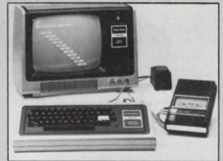
The latest home computer, the TRS-80 from Radio Shack, uses a Z-80 micro. It comes assembled and tested with Basic language in ROM for $599.95.
