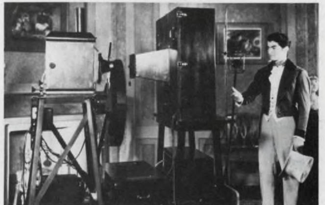
1928—"And now, station W2XBS presents..." Experimental broadcasting (over wire) didn't wait for such "unessential" items as pickup and picture tubes, amplifiers, and other electronic circuitry.
