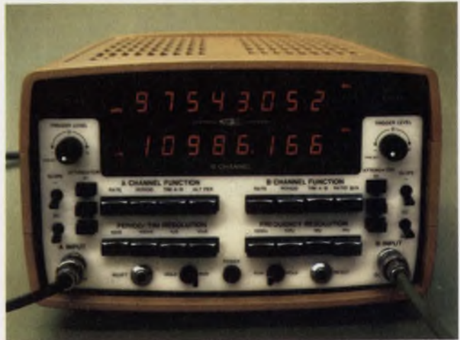
The first dual UCT, the 6361A from Systron-Donner, takes advantage of recent LSI advances to package two independent channels, each with its own display, under one roof. The 100-MHz unit sells for $895.
