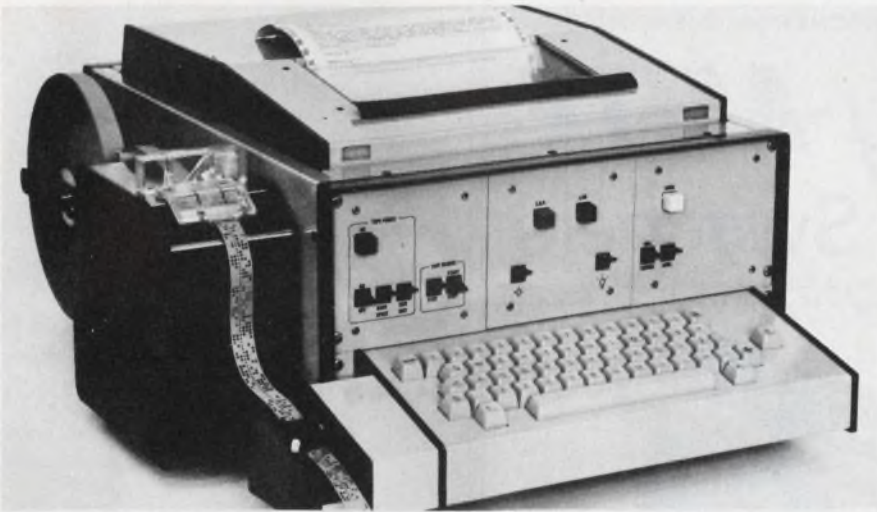
Two-way printing and a dot-matrix head made this teleprinter multilingual.
