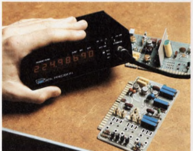
The 585 portable frequency counter marks Data Precision's first entry into the field. The eight-digit, 250-MHz unit works from NiCd batteries.
