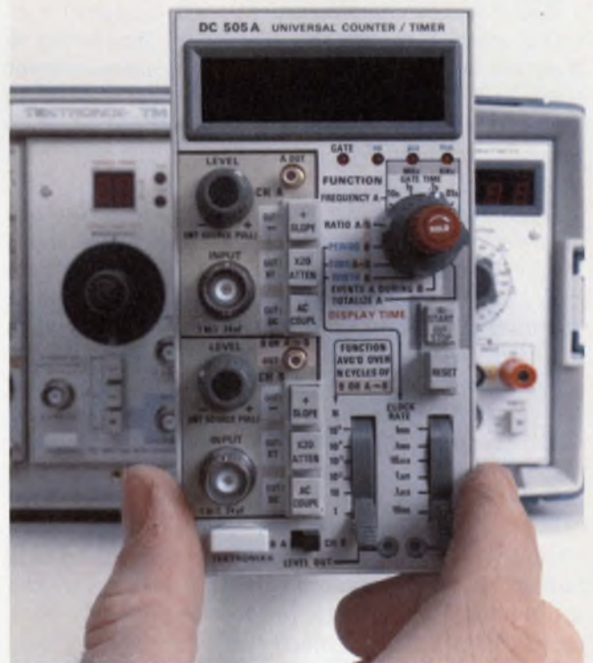
Combine a counter and an oscilloscope and you can make otherwise difficult measurements. The Tektronix DC505A UCT can read out a selected portion of the waveform displayed on the scope.
