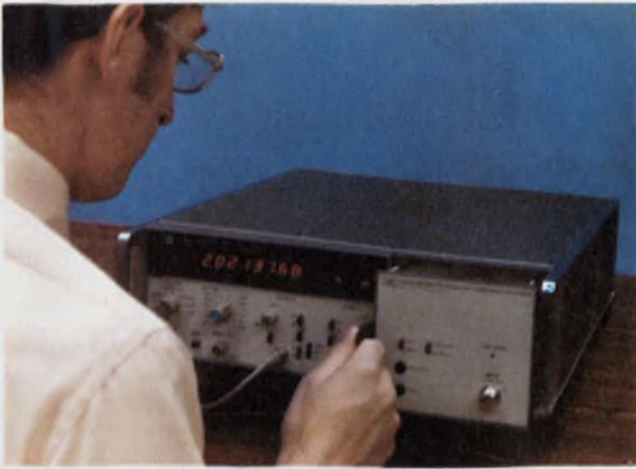
Dc-coupling to 500 MHz with 20-mV rms sensitivity: The top-of-the line Hewlett-Packard 5345A is the only counter that can claim those specs.
