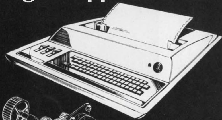
Schematic showing motor drive arrangement. A pinion mounted on the motor shaft engages a spur gear that drives the carriage platen.
