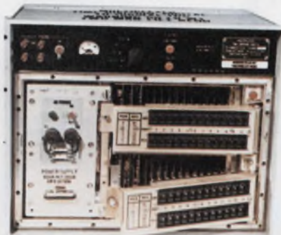
The TD-1069 Time Division Multiplexer (TDDM) multiplexes and demultiplexes up to 24 separate digital and teletypewriter dc signals into a bit stream of 32 Kbp/s.
