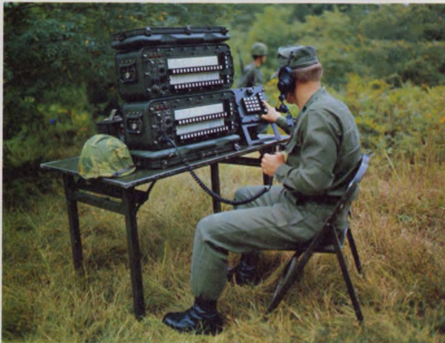
The Army version of the Marine Corps SB-3614 switchboard provides fully automatic queuing, ring and disconnect. It is built by Sylvania.
