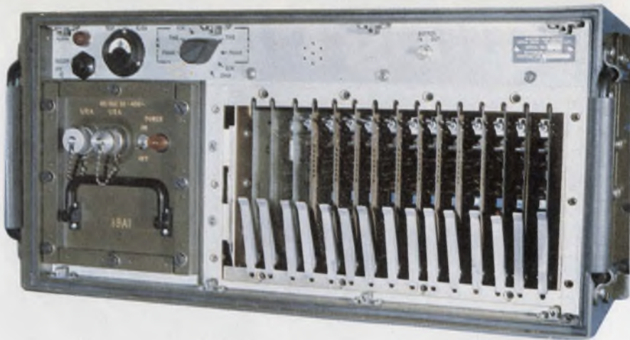
High-Speed Data Buffer TD-1065 is being developed for digital access of high-speed data and wideband, secure voice traffic at rates of 32,000 and 16,000 bits/s into the Army's tactical trunking system.
