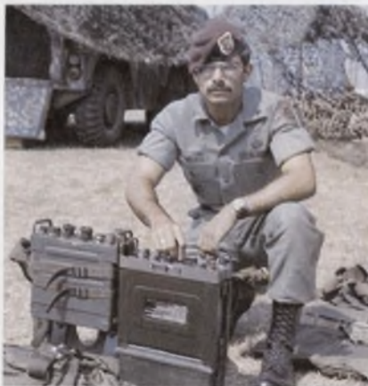
The AN/PRC-77 manpack radio , which still uses some germanium transistors, will be used until Sincgars radios come into inventory.
