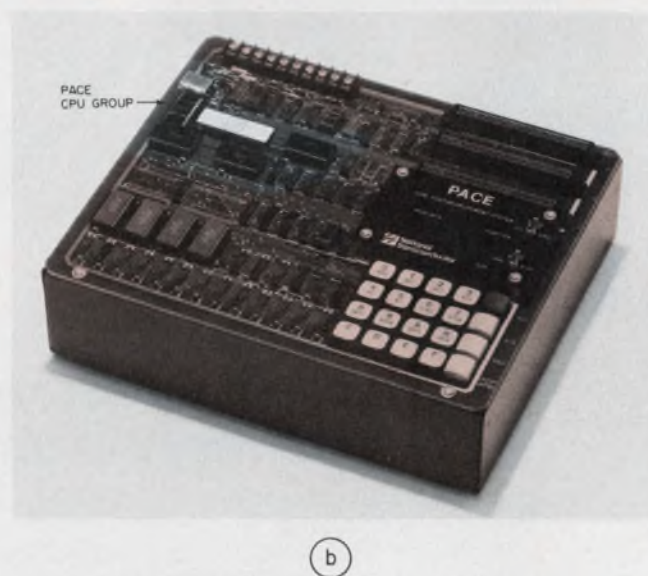
1. A minimal operating system can be built from the PACE, three BTEs, one STE and any amount of RAM or ROM (a). All input/output lines of the system can handle 30 TTL loads. A simple development system (b) uses three BTEs and simple TTL. Either the self-contained keyboard or a teletypewriter can be used.
