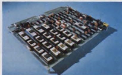
The EVK 300 from AMI is one of a series of four PC boards for designing 6800-based systems.
