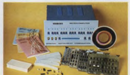
Designing with the 16-bit CP1600 \mu P is made easier by General Instrument's Gimini microcomputer.
