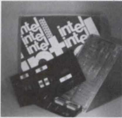
Intel's SDK-80 is a complete 8080 microcomputer on a single PC board. Instruction-cycle time is 2 \mu s.
