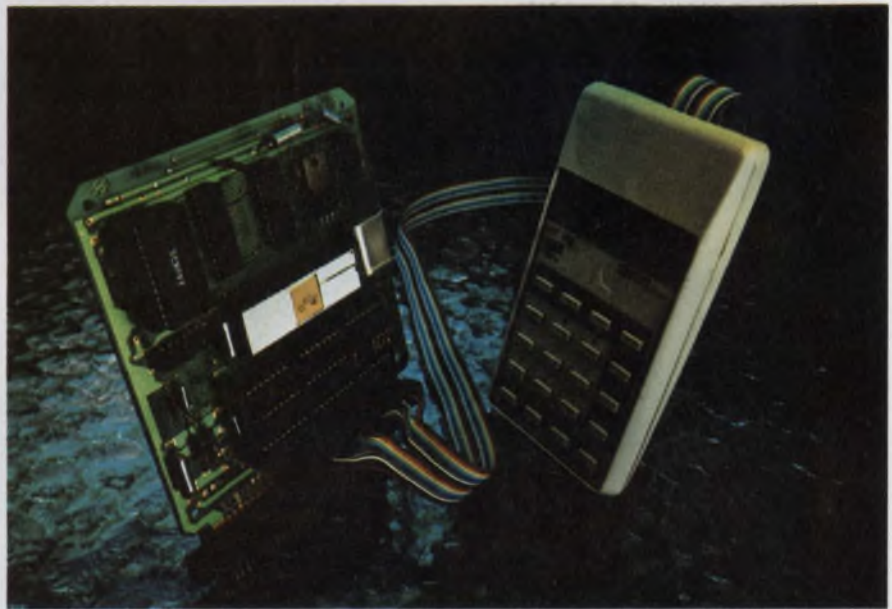
Input/output capability at low cost for National Semiconductor's SC/MP kit is provided by a hand-held hexadecimal keyboard and display. A 21-wire flat cable supplies the connection to the \mu P board.
