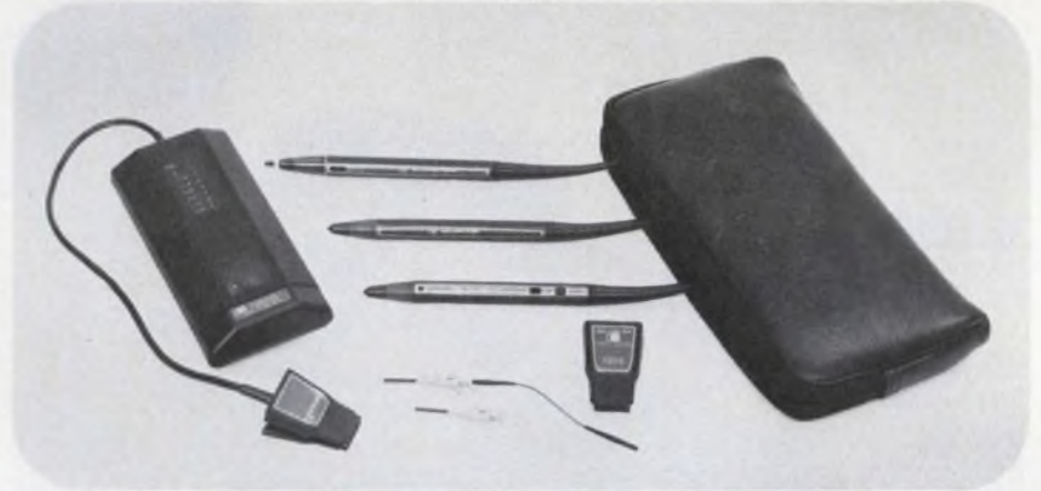
The HP 5023A shown here contains all five new IC troubleshooters from Hewlett Packard. Three kits are now available, each packaged in a convenient zippered vinyl case.
