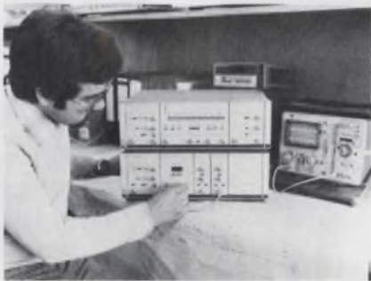
This is a pulse generator.
