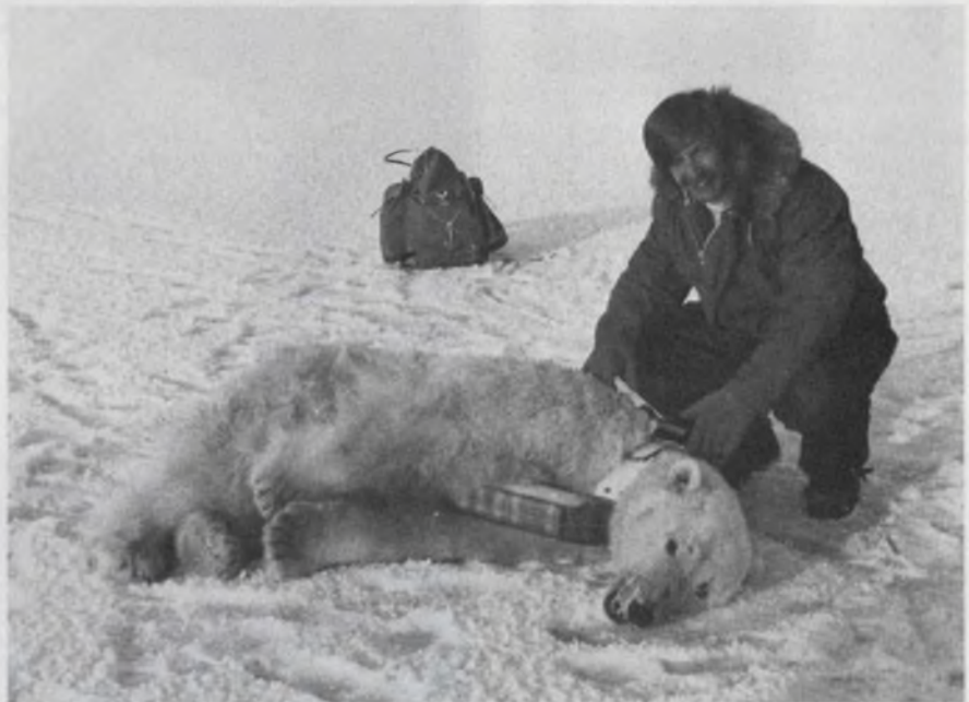
A miniaturized telemetry package that is strapped on to polar bears in Alaska relays a bear's location to researchers via the Nimbus weather satellite. Scientists are studying the effect of the Alaskan pipeline on hibernation patterns.
