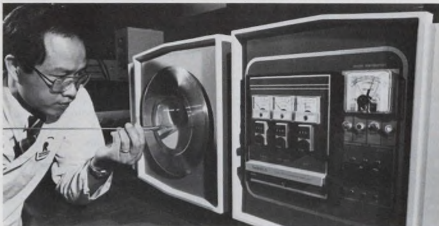
Laser crystals made of lead-tin-telluride are being grown at General Motors for use in pollution monitoring systems.
