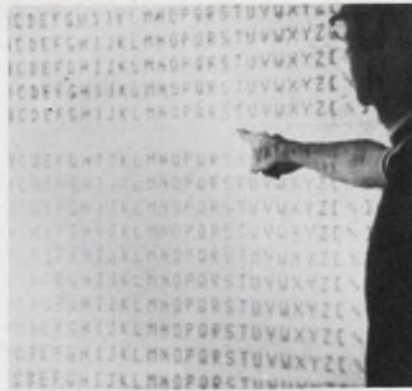
Dr. Lee T. Todd, Jr., inventor of MIT's CCRT tube, shows the selective erase capability of a projection tube display.
