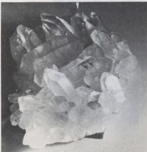
Before World War II, Brazilian natural quartz was employed for most oscillator crystals. Now artificially cul-
