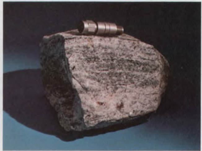
Rock-stable miniature attenuators are produced by Engelmann Microwave. They are good up to 18 GHz, have SMA connectors and use a pyrolytic deposition process to put down carbon film resistors on heat-conductive ceramic cores.
