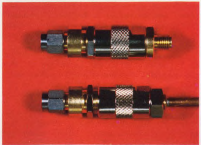
A connector with a built-in line stretcher is the Phase Adjustable SMA from Amphenol. The connector comes either as an individual component or as a cable terminator. VSWR is better than 1.28:1 up through 18 GHz, and the phase can be adjusted by 10^\circ times the frequency in GHz. Thus, at 10 GHz, the phase can be adjusted up to 100^\circ .
