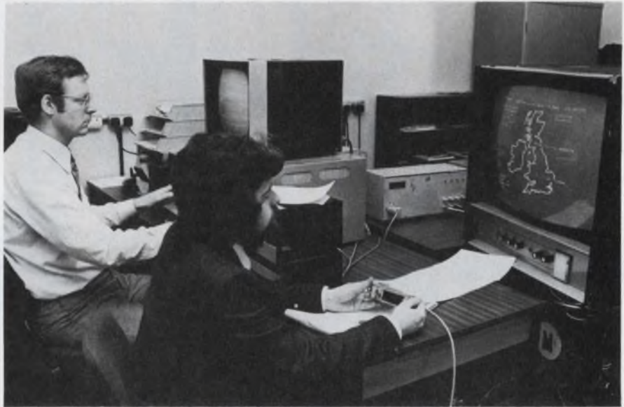
Updated information is being entered into the CEEFAX system via computer terminal (upper left), while a TV monitor shows a weather map that is being transmitted (lower right).
