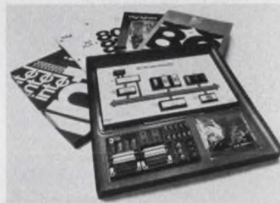
A complete system based on the 8080A can be built with an Intel kit priced at $350.
