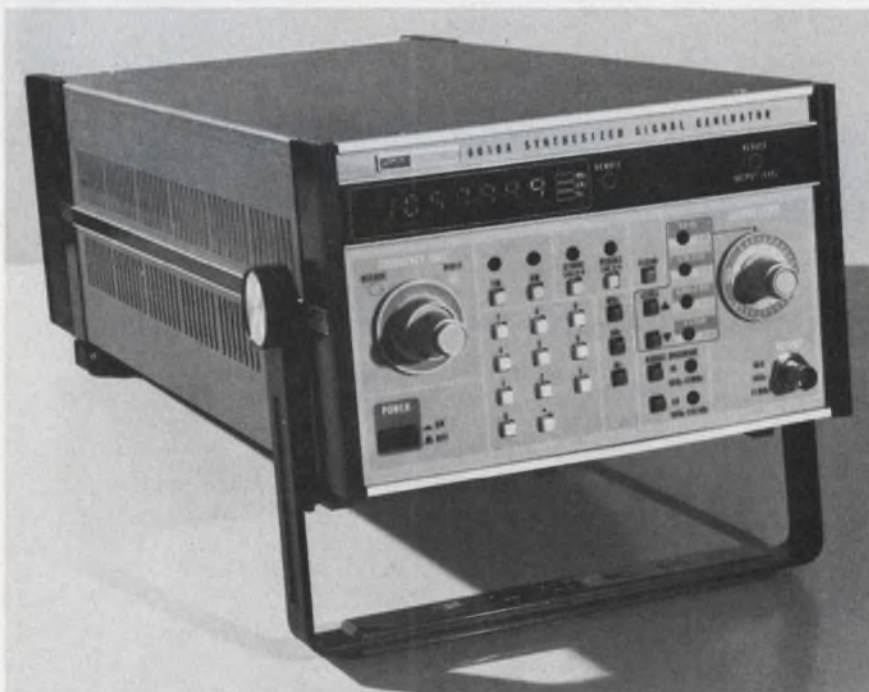
The new look in synthesizers: numeric keyboard entry of frequencies, the ability to store and recall frequencies at the push of a button, and other features—all made possible by the LSI microprocessor.
