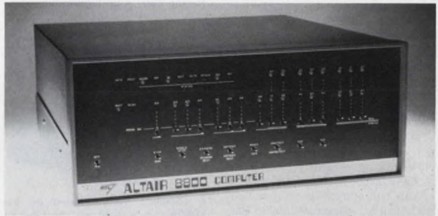
The unit that started the current popularity in kits—the Altair 8800 from MITS—is based on Intel's 8080 \mu P. One reason for the kit's acceptance: Programming can be done in Basic.
