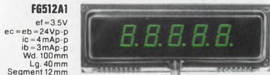
Instruments & Terminal Units Display
