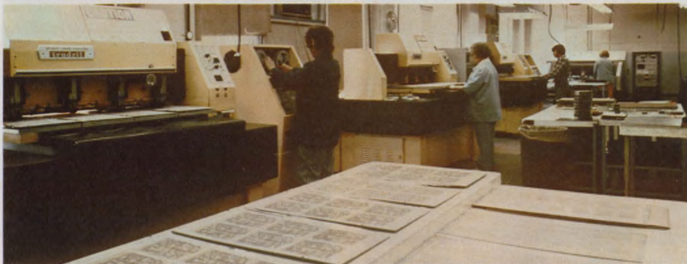
Numerically controlled drills at the Bureau of Engraving, Inc., handle panel sizes to 25 × 25 in. Taped data
