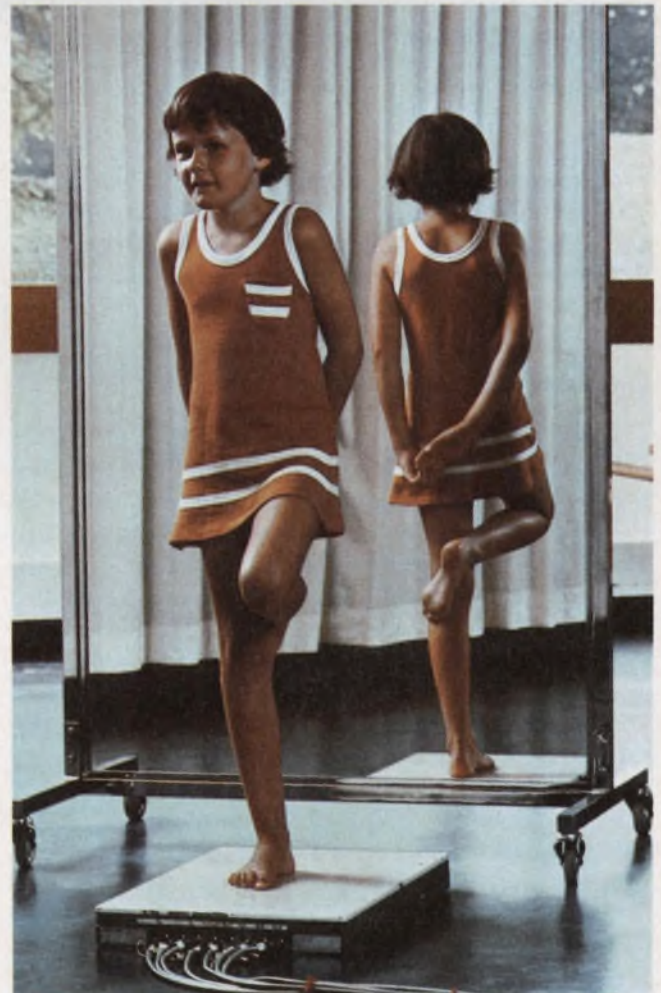
Bioforce tables , designed by Kistler, can evaluate the component forces in prosthesis loads, posture control, optokinetic effects and gait analysis.
