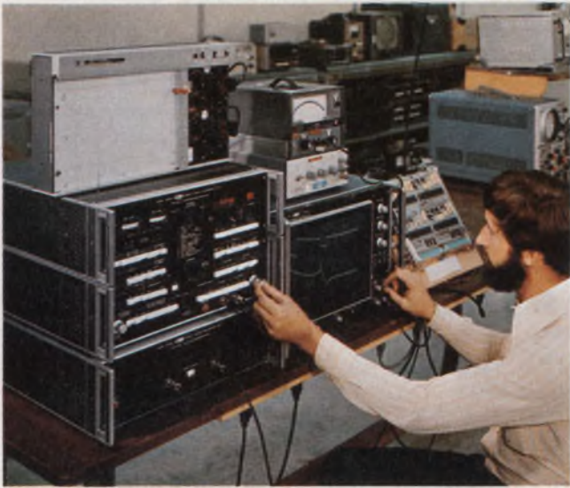
A complete stand-alone FFT processor with 15 built-in programmed calculations can analyze two signals simultaneously. The SD 360 from Spectral Dynamics shown here can perform cross-correlation and display probability-density histograms.
