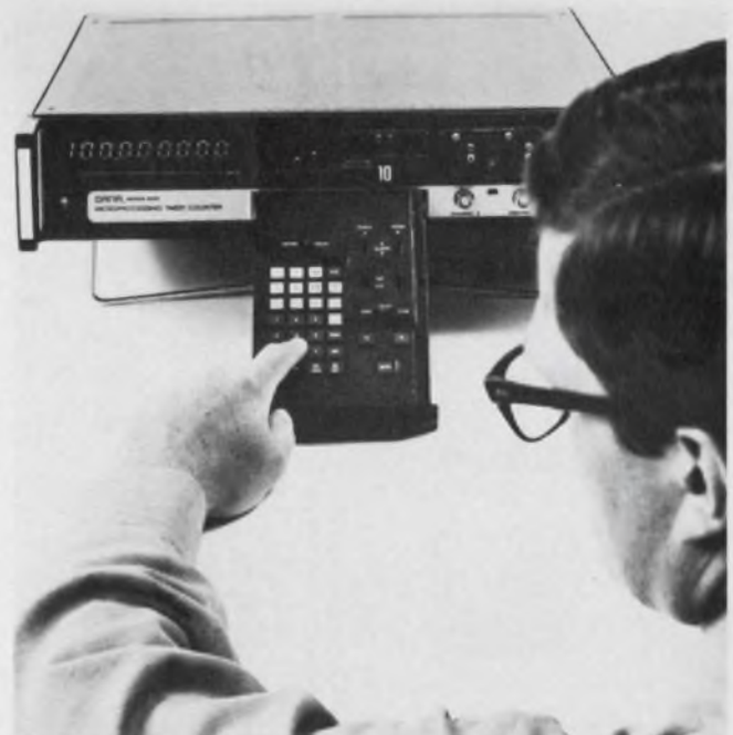
The Series 9000 counter/timer from Dana uses a microprocessor to provide automatic triggering and calculate rise and fall times.
