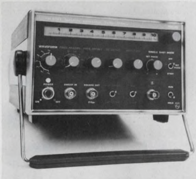
The PM5167 function generator delivers signals over a 0.001-Hz-to-10-MHz range and has a linear dial indicator to make tuning easy. It is made by Philips.
