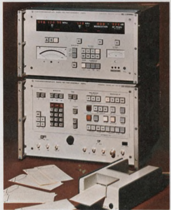
Twelve pieces of equipment can be replaced by this microprocessor-controlled radio-set test assembly from Rohde & Schwarz. It can automatically test for bandwidth, sensitivity, squelch response and signal-to-noise ratio.
