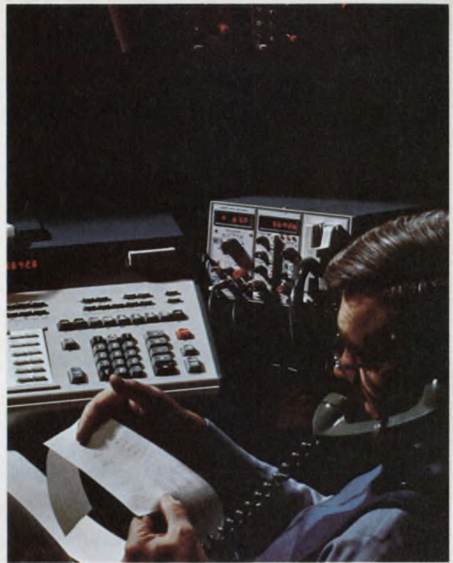
A magnetic tape cartridge in the Tektronix 31/53 calculator provides automatic data acquisition, logging and statistical routines for interchangeable plug-in modules.
