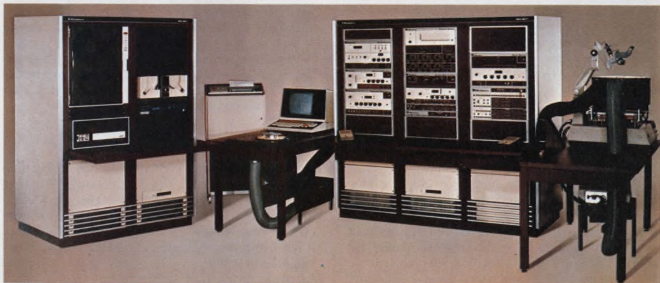
Using a microprogrammable multiprocessor approach, the Macrodata 501 performs functional and dc/ac para-
