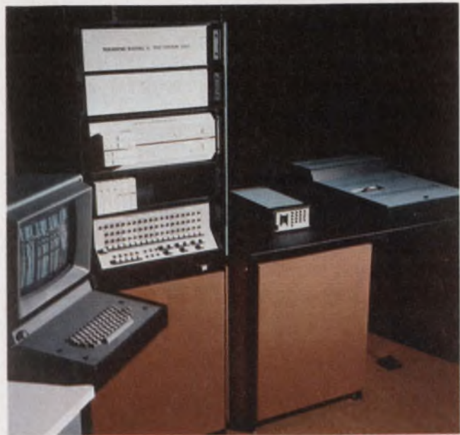
Teradyne's J325 digital IC tester accepts up to four test stations. Devices handled include ECL, TTL, DTL, CMOS and static MOS. Data logging, summary reports and Schmo plots are part of the unit's capabilities.
