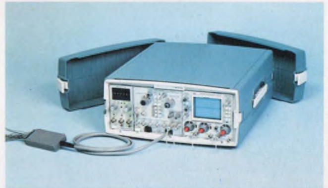
The LA 501 Logic Analyzer from Tektronix works with any CRT display. It displays up to 16 channels of data in a timing-diagram format and contains 4096 bits of storage. The unit is a plug-in module.
