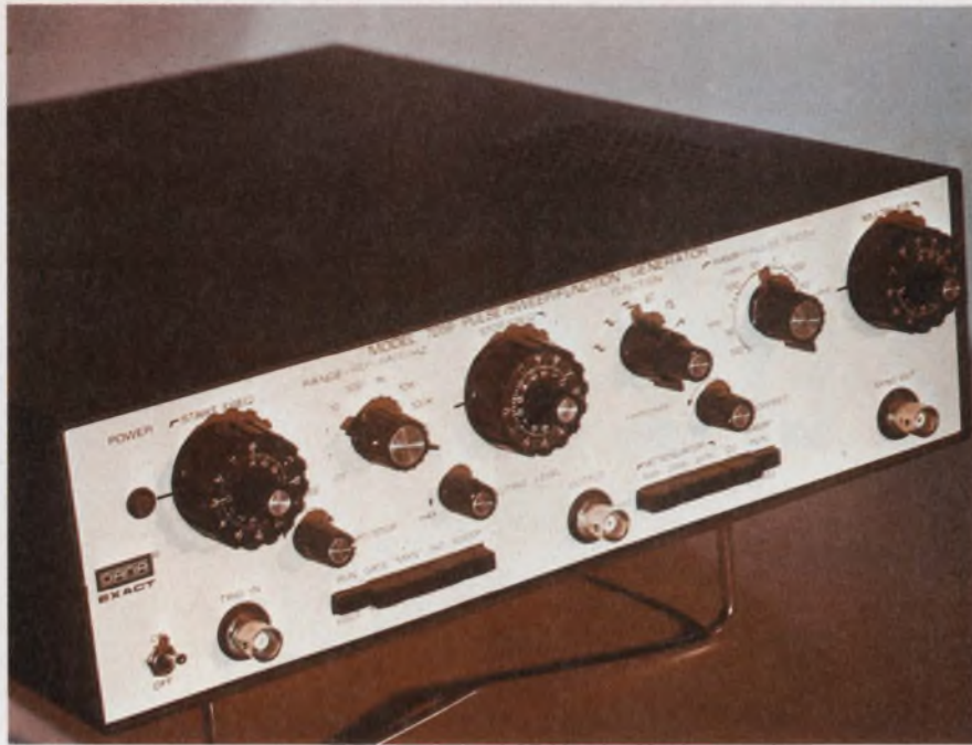
The Model 7059 from Dana/Exact offers pulse, sine, square, triangles and swept functions all in one compact instrument.
