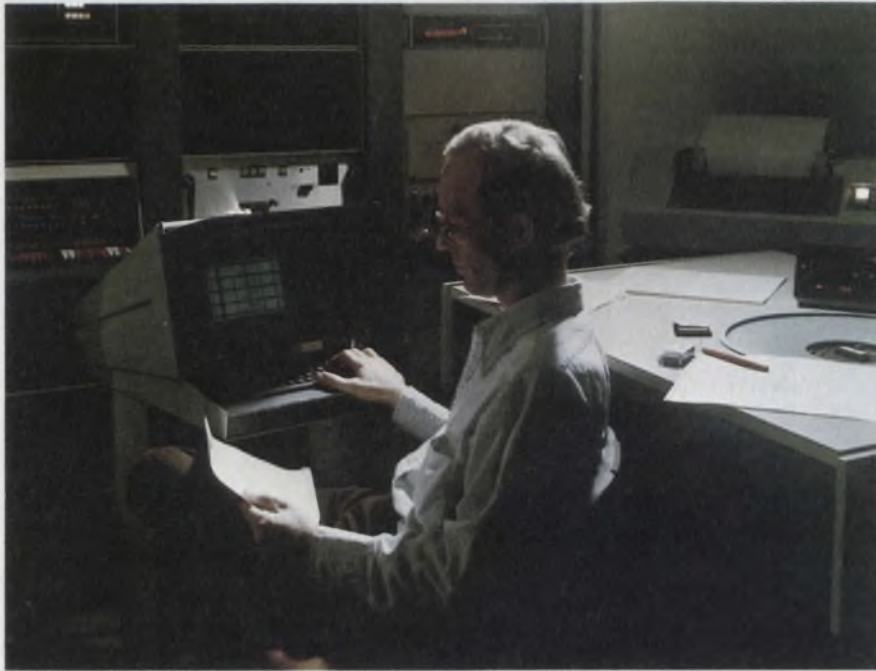
One burning test issue today: How to test a microprocessor. Here the Tektronix 3260 generates and edits test patterns on the Intel 8080. Sector cards are the key to pin control.
