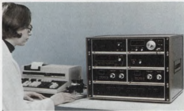
A test setup for measuring semiconductor parameters uses the Keithley System 1 instrumentation, controlled by a modified version of the Monroe 1880 calculator.
