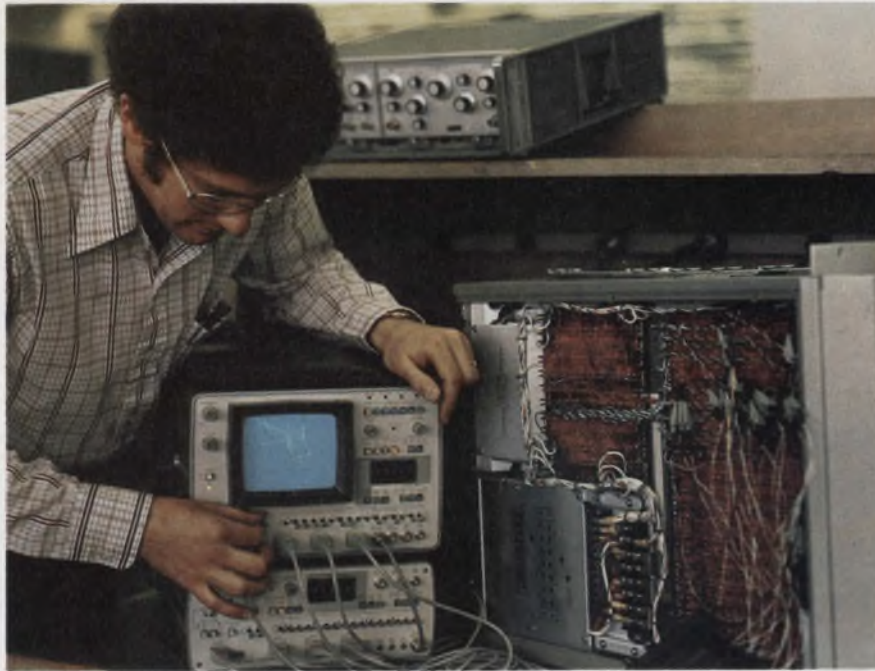
A unique mapping mode is available with the Hewlett-Packard Model 1600A Logic State Analyzer. Digital words are presented as dots on the display, each word having a unique position. Vectors trace the digital sequence from word to word. It works with up to a 20-MHz clock.
