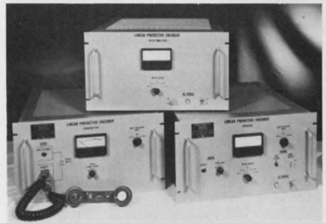
Special speech scramblers, called linear predictive encoders, are used by the military to provide secure communication between two points. These devices were built by ITT for use by the Navy.
