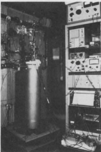
Superconducting magnetometer uses Josephson effect for ultrasensitive measurements.
