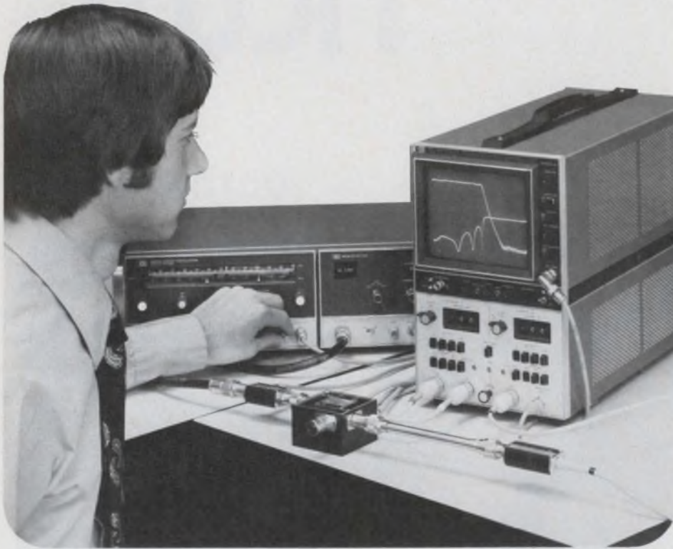
"Hardware"—New reflectometer bridge for HP 8755 test set brings convenience and precision to broadband measurements.
