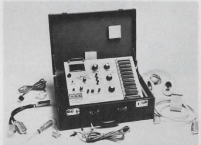
Bugs and taps can be detected and eliminated with telephone analyzers, such as the TA-17 from Communication Control Corp. It can check for tone and voltage activated devices, as well as hook-switch bypasses.
