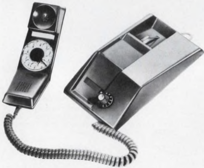
"Tap-proof" telephone from Communication Control really isn't. While it does detect most bugs and wiretaps, there are still some that it doesn't catch. The phone indicates that a conversation is not secure by sounding a buzzer or disconnecting from the circuit.
