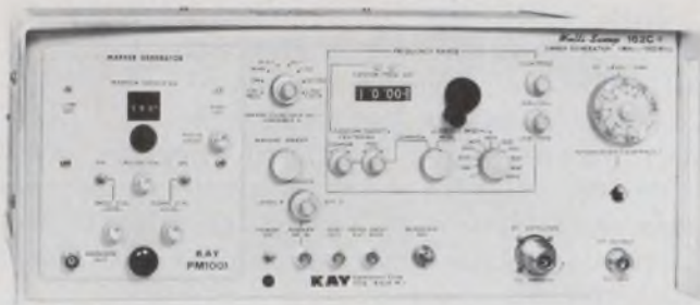
The 162C is Kay Elemetrics' wideband, 1-to-1000 MHz generator. A summation sweep mode is offered as an option to test CATV amplifier trunk lines.
