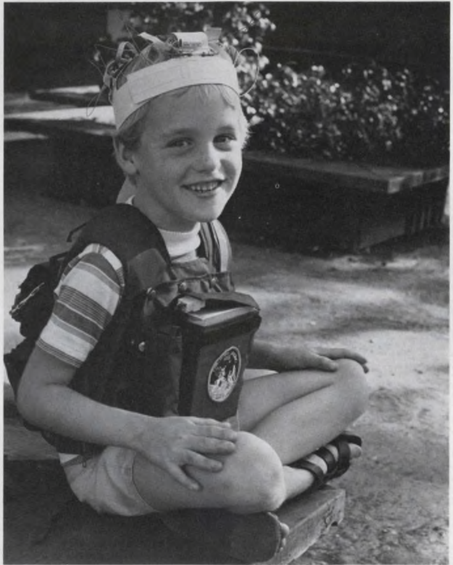
EEG digital monitoring of epileptic children will be done with this system from Stanford Research Institute. Scalp electrodes feed four channels of EEG data to a data-acquisition system in a lightweight vest worn by the child.
