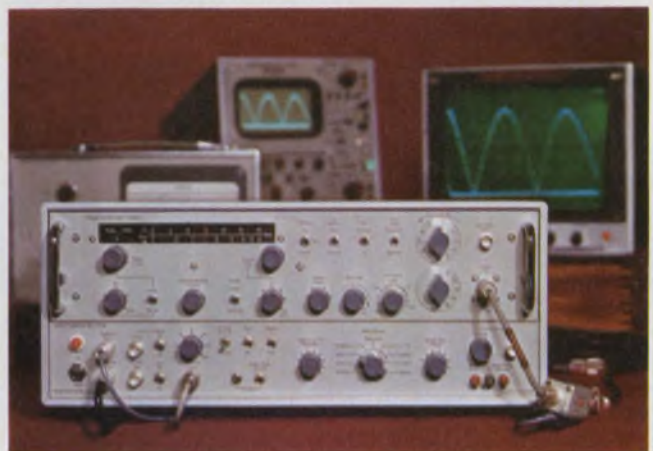
Various plug-ins for the TF2361 sweep generator—backbone of the Marconi line—convert the unit from a general purpose to a specialized instrument. Shown is the video plug-in: 25 kHz to 30 MHz in one sweep.
