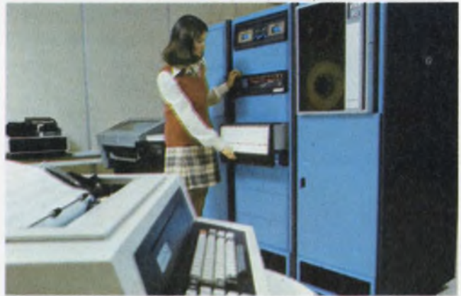
A 32-bit minicomputer with 1 Mbyte of core cycles at 450 ns average, 300 ns minimum. Interdata's 8/32 Mega-mini uses high-speed Schottky-TTL circuits.
