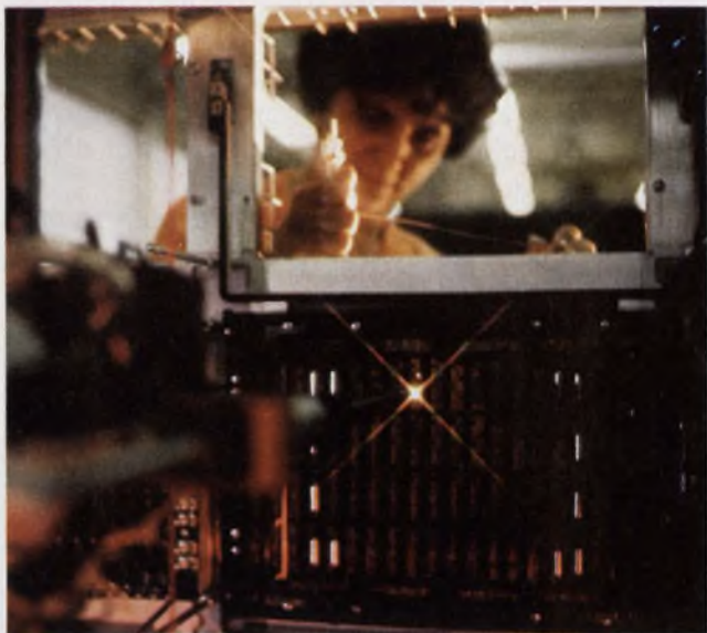
A computer-directed halo of light shines through a PC board and shows an assembler where to place the next wire. The computer then tests the connection (IBM).
