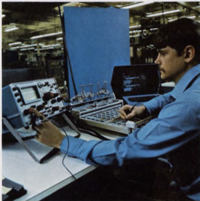
Computerized checkout of an Interdata 7/32 minicomputer processor board. The terminal displays input data plus expected and actual output data.
