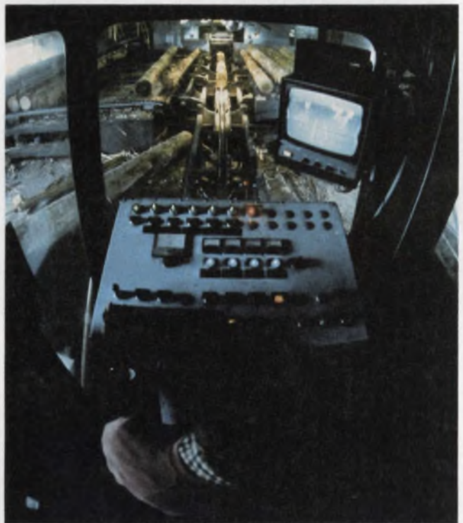
As logs are measured in a sawmill, a PDP-8 tells an operator of a four-blade saw which sizes and lengths to select to get the maximum yield of usable lumber.
