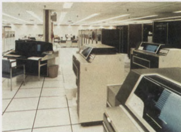
Service centers with multiple computer systems form the backbone of Control Data's Cybernet. The computer network offers time-sharing access to design programs on user terminals, as well as allowing user computers to augment their processing power with the network.
