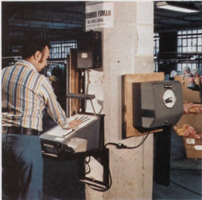
This security system uses the unique geometry of a human's hand to verify or deny entry to employees at My Toy Corp. The handprint is scanned by an Identimat machine and is compared with the digital description on a magnetically encoded card.
