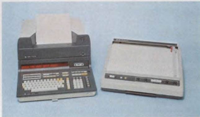
The arithmetic prowess of programmable calculators makes them a natural for CAD. HP's 9830A (left) executes a comprehensive microwave design program called BAMP, and Tektronix offers microwave software on its
