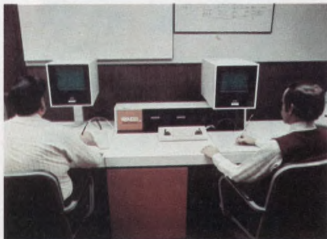
Computer-aided designs often start with a spec and end with complete PC board layouts. RCA uses Applicon graphics terminals to master the layout problems associated with complex MSI and LSI components, after CAD programs verify the design.
