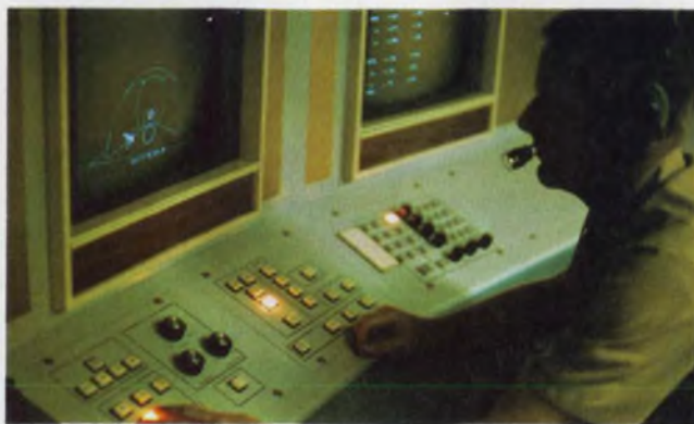
A dogfight flight training system for the Navy pits pilot against pilot in mock air-to-air combat. The computer-based system, by Cubic Corp., provides mission replay.
