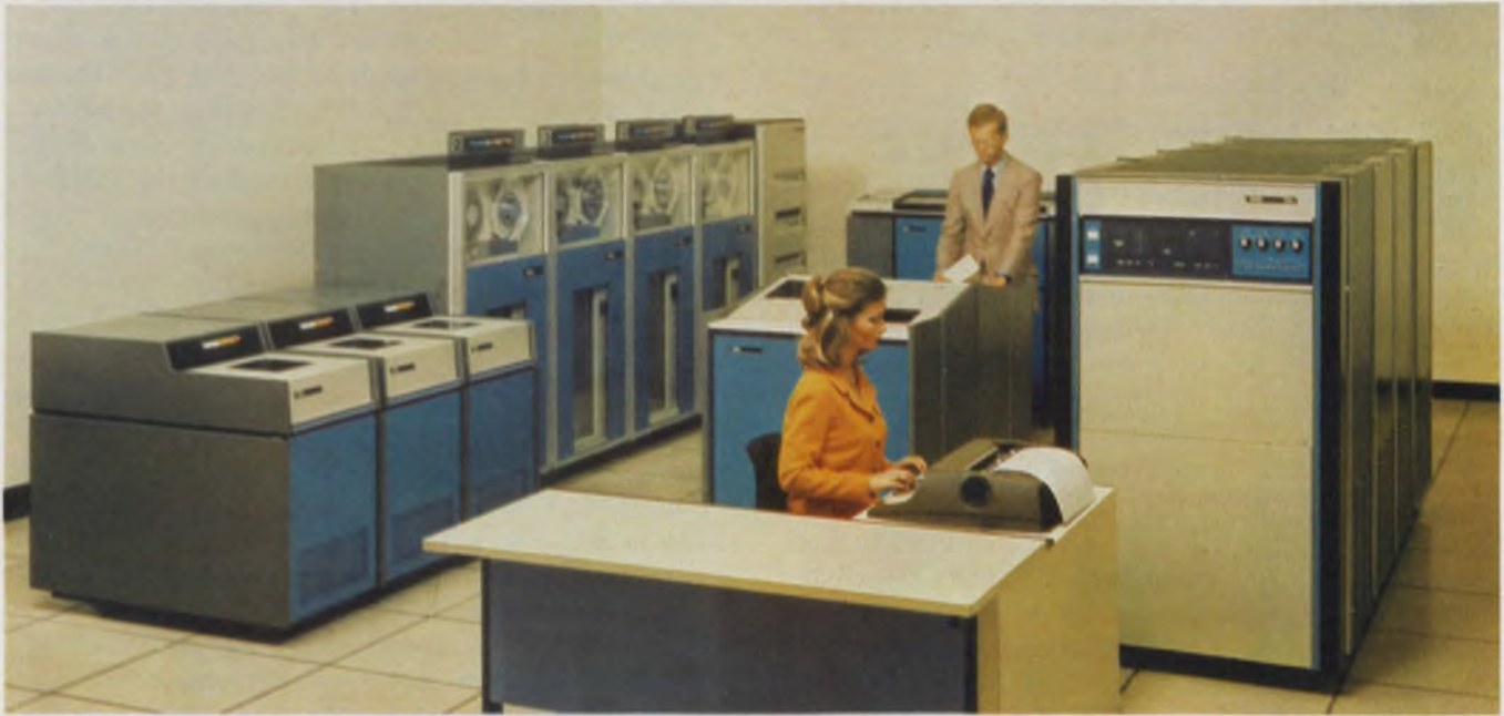
A single system processor controls input/output and arithmetic processors in the hierarchical architecture of the Xerox 560 computer, a 32-bit mini. Independent
