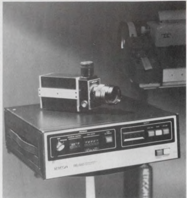
Digital cameras can feed data to computers so that noncontact inspection, process-control and size and position measurements can be made. This system—the LC600—is from Reticon.
