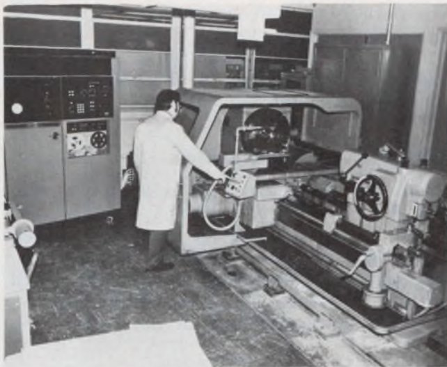
Computerized numerical control , as represented by GE's 8500 Series, provides a programmable and solid-state output to previously relay-sequenced machines.
