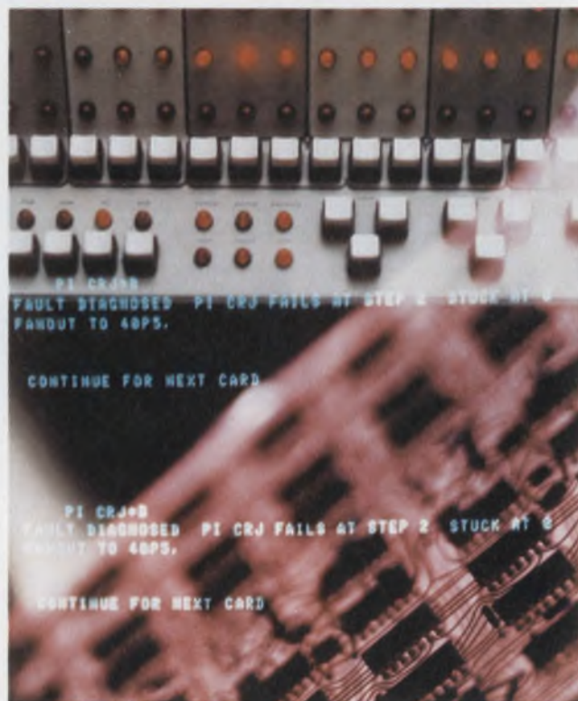
Diagnosis by computer: Teradyne's L100 automatic test system checks arithmetic boards for the company's M365 computing controller, and it pinpoints any faults.
