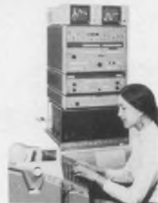
FFT Analyzer with add-on mini-computer for post-processing.
