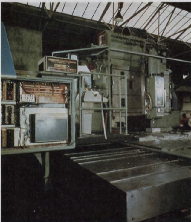
A large milling machine is controlled by a PDP-14 mini-computer at the Toulouse factory of Aerospatiale, France's largest aircraft maker.
