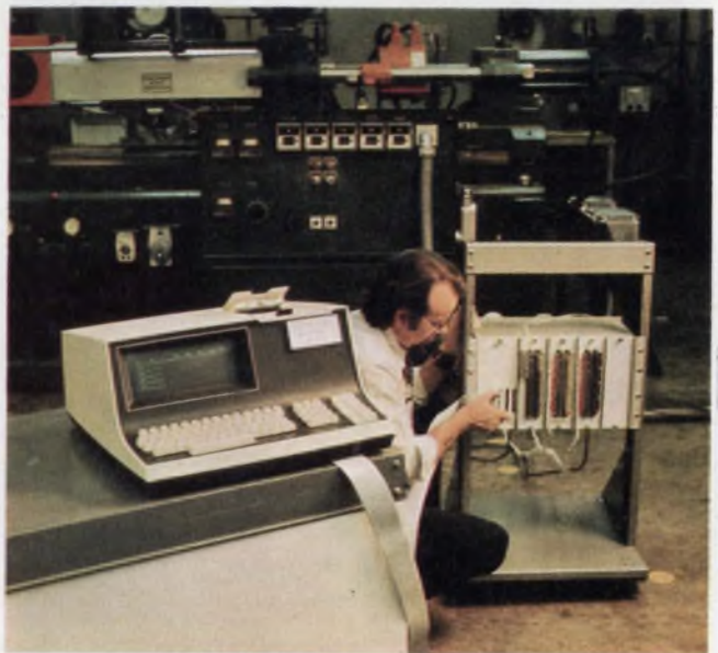
Programmable controllers, such as this Eagle-Signal CP600 with solid-state circuitry, are replacing the conventional relay-sequencing controller.
