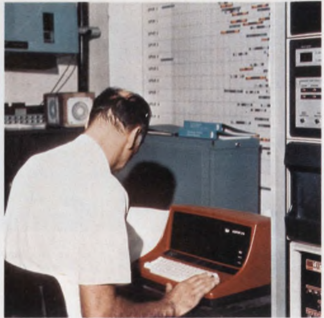
An instant check on baggage handled by the automated system at Eastern Airlines' Miami Terminal is made at the computer. The DEC computer, laser optical readers and conveyors are linked in this Bendix system. The optical baggage tag is a coded bullseye.
