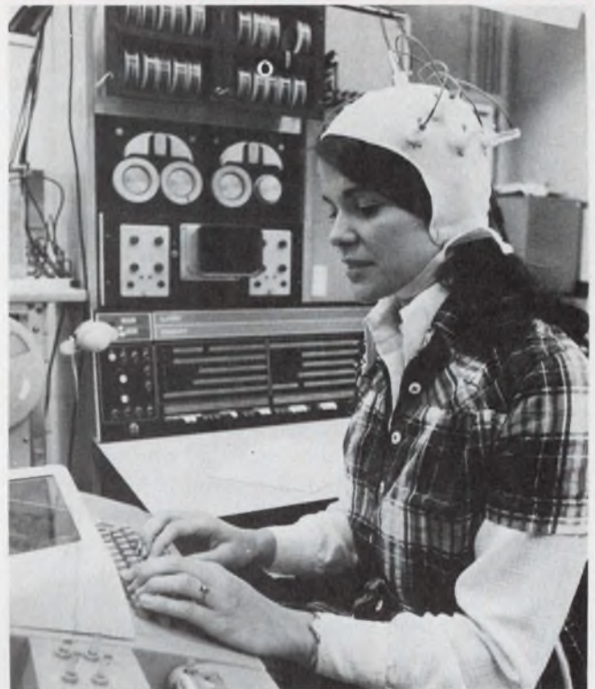
Brain-to-computer interface system being developed at Stanford Research Institute allows a person to enter data into a computer by "thinking" it in. Accuracy and system vocabulary have to be significantly increased to make thought input a viable method of entering data into a computer.
