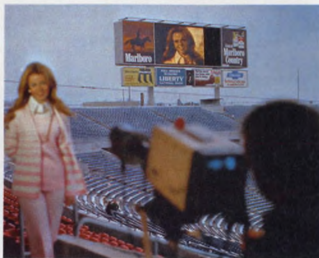
Pictures from a local portable TV camera or from network stations are processed by computer and projected from a computerized football scoreboard by Conrac.
