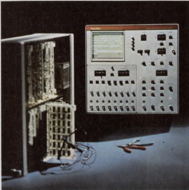
Logic analyzers form a new class of test instrument to meet the needs of digital-logic troubleshooting. The main features of the class include the ability to display many
