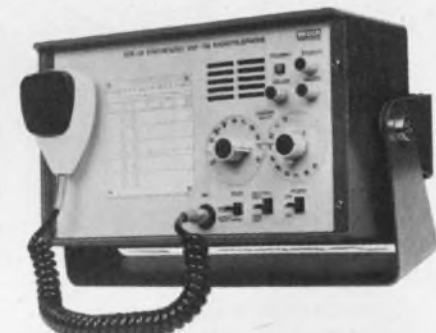
Vhf/FM radiotelephone covers all channels, including 16 with a single crystal. Priced at $1475 by ITT Decca.
