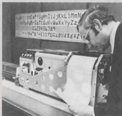
Non-impact tactical line printer is examined by engineer at RCA's Advanced Technology Laboratories.
