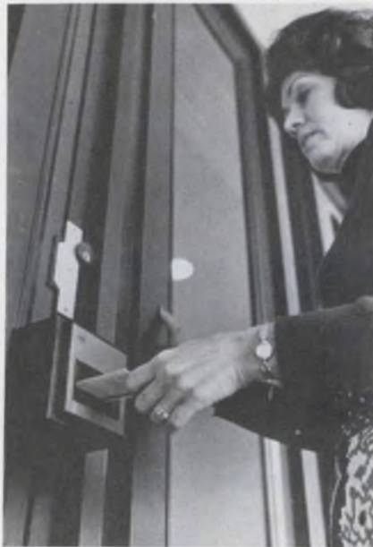
Magnetic cards can be used to control access to computer facilities.
