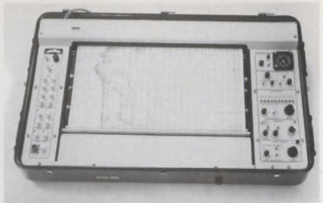
Electrosensitive recording paper with a 23-dB tonal range from white to black is used in the EPC line to provide a facsimile-type presentation.
