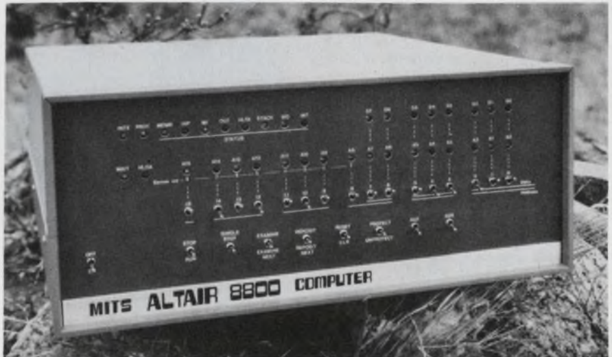
The Altair 8800 computer kit uses Intel's 8080 processor and is said to offer performance equal to that of computers costing six times more.
