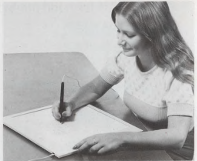
3. A standard data-tablet system with a preprinted overlay sheet serves as the input to the character-recognition system.
