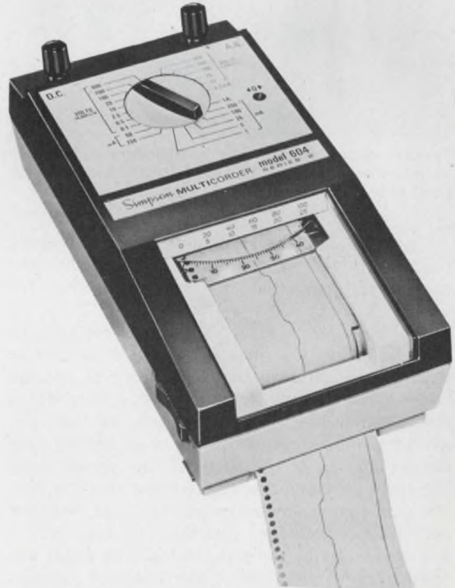
The Simpson 604 Multicorder can be likened to a multimeter with a recording device instead of a meter. The unit measures volts, amps, millivolts and milliamps.
