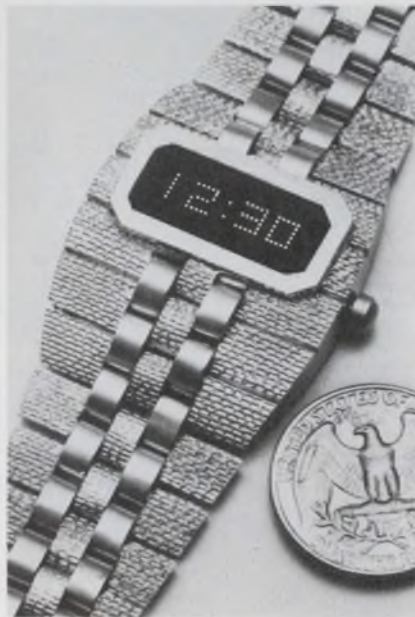
New SOS and I 2 L watch technologies will compete with present CMOS designs. This Accuquartz, by Bulova, has a 78.6-kHz crystal and a LED display.
