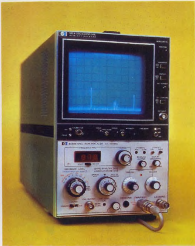
That analyzers are getting easier to use is demonstrated by Hewlett-Packard's 8558B. Just three controls are needed to make practically all measurements.
