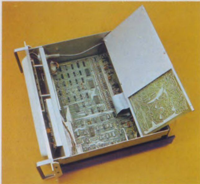
Dc logic switching in the Philips PM 3260 120-MHz oscilloscope provides more efficient placement of operator controls. Simplified servicing is an added bonus.
