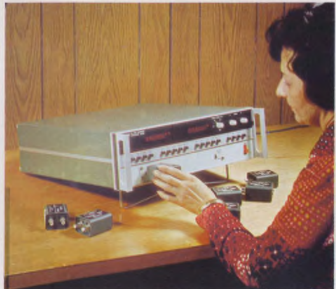
A microprocessor in this automatic capacitance bridge, by Boonton, eliminates the use of error-correction charts by calculating and compensating for instrument errors.
