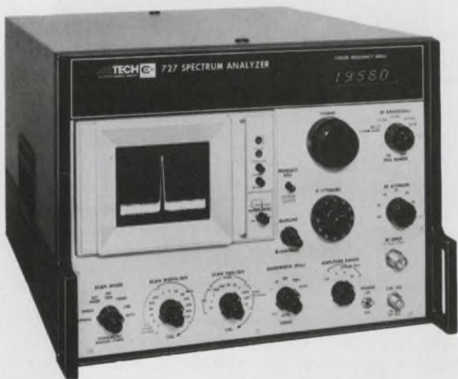
Recently unveiled at Wescon, this unit from Ailtech offers built-in YIG preselection out to 20 GHz. Outstanding is the unit's 100-dB dynamic range and 5:1 shape factor.
