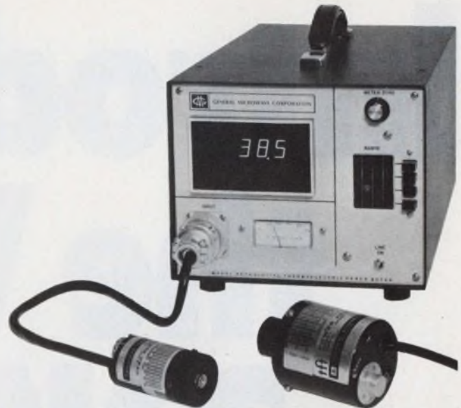
Direct reading from 10 nW to 3 W on a digital display is possible with the Model 467A meter from General Microwave. The unit employs a thermocouple sensor.
