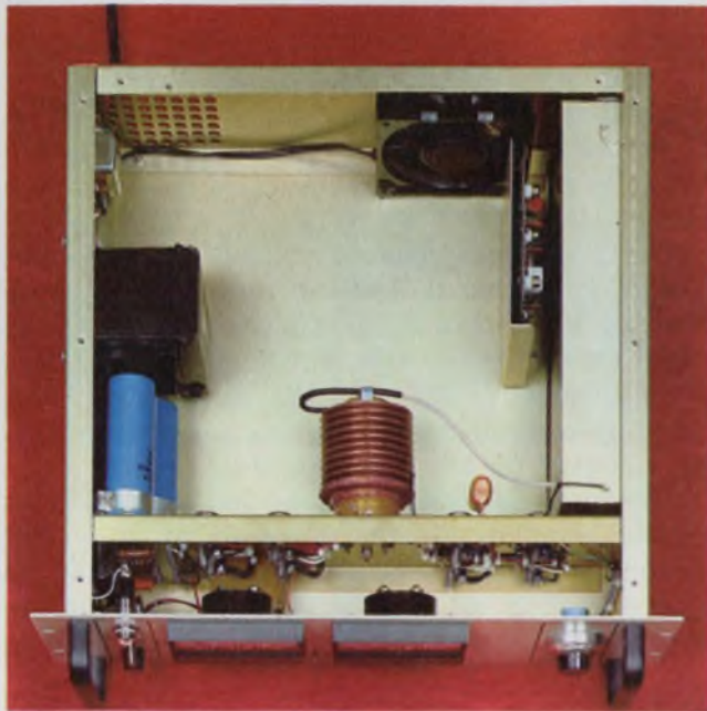
High-voltage laboratory power supplies, like this model RHR40P120 from Spellman High Voltage Electronics (top), are not made to fit the smallest space. Inside the unit (bottom) open space is needed for cooling.
