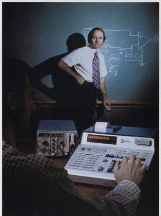
Under control of a Tektronix 31 programmable calculator, the 31/53 system can process data from a variety of instruments in the TM-500 series of plug-in devices.
