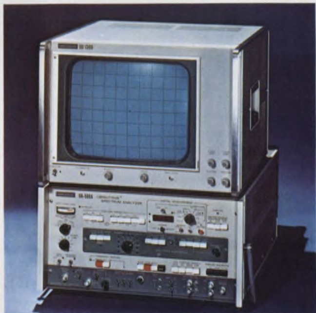
Real-time analyzers use digital algorithms to perform a Fourier-transform analysis of incoming signals. The unit shown is Nicolet Scientific's UA500A, an analyzer that performs digital calculations.
