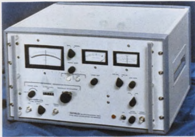
Attenuation calibrator spans the broad range of 10 MHz to 40 GHz. The Model 915-B from PRD (Syosset, NY) measures up to 110 dB in a single step and accepts levels as low as -120 dBm.
