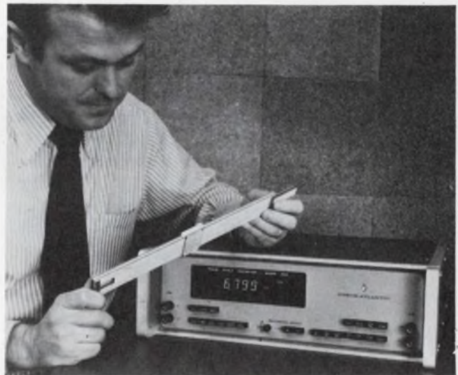
The first digital phase angle voltmeter is the 225 from North Atlantic Industries. A ratio-metric option displays ratio of input to a reference.
