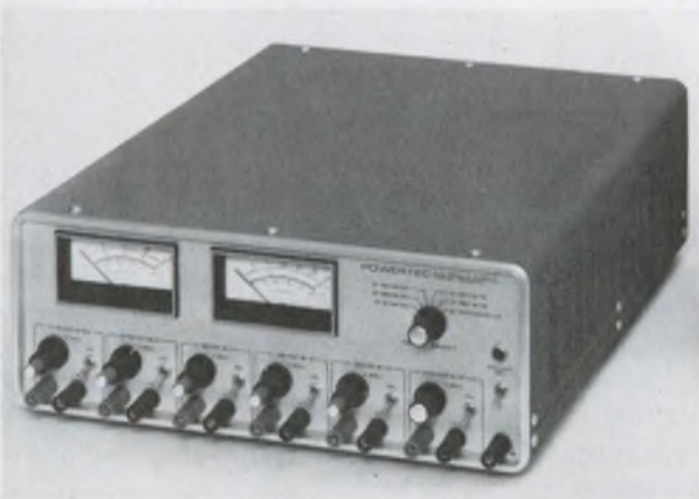
One of the most versatile units is the 6D6000 made by Powertec. This unit delivers six variable outputs.
