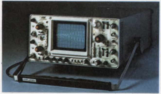
The fastest storage scope around is the 466 from Tektronix. It has a writing speed of 1350 cm/ \mu s and a viewing time of from 15 s to 6 minutes.
