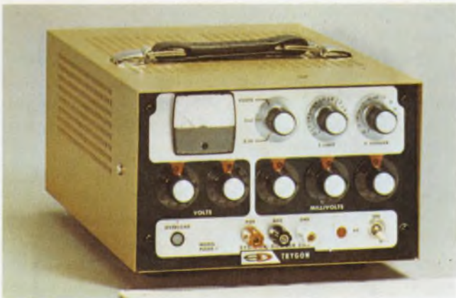
For precision power, calibrated laboratory power supplies use digital readout switches and resistive dividers to deliver levels with millivolt accuracy. This unit is from Trygon.
