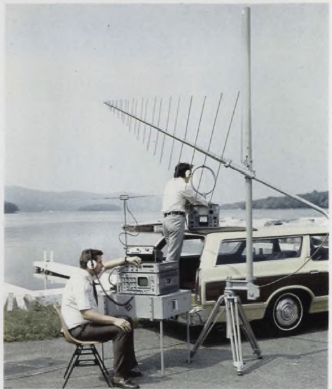
Battery operation for field use is another trend in spectrum analyzers. Though it can be used outdoors, Rohde & Schwarz's Analyoskop gives laboratory performance.
