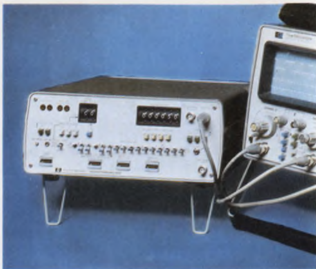
Pattern analyzers that trigger scopes on the occurrence of a specific bit pattern, are becoming popular because they provide jitter-free traces.
