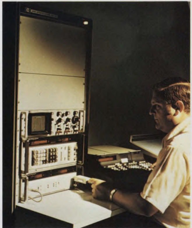
The first system to use the HP Interface Bus is the 3042A network analyzer from Hewlett-Packard. This system is a calculator-controlled frequency synthesizer and network analyzer for measuring amplitude and phase from 50 Hz to 13 MHz.
