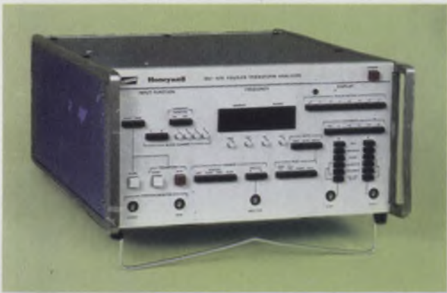
Dual-channel analysis is performed by Honeywell's SAI-470, an instrument that exemplifies the newest trends: RAMs, LED readouts, digital circuitry.
