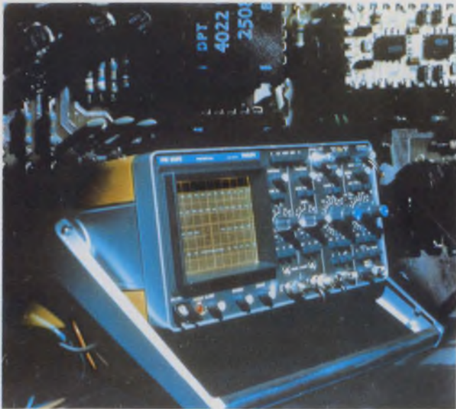
The use of dc logic switching in this Philips PM 3260 120 MHz oscilloscope provides more efficient location of operator controls. Simplified servicing also results.
