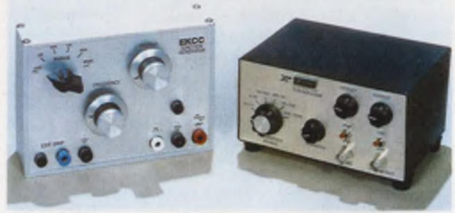
A two-chip monolithic waveform generator is incorporated in the prototype instrument by Exar, at right. A single-chip device is used in the other instrument, produced in kit form by Electronic Kits and Components.
