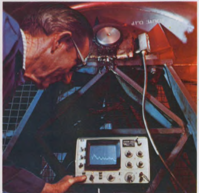
Clear, steady displays of slow sweeps are possible without storage tubes. The secret? Refresh the display at high speed from a digital memory as does this unit from Hewlett-Packard, the 3580A.
