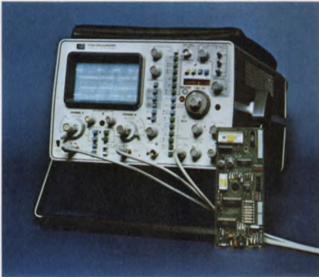
Oscilloscopes are getting smarter and the latest entry is the 1722A microprocessor scope from HP. It uses the micro from the HP-35 calculator.
