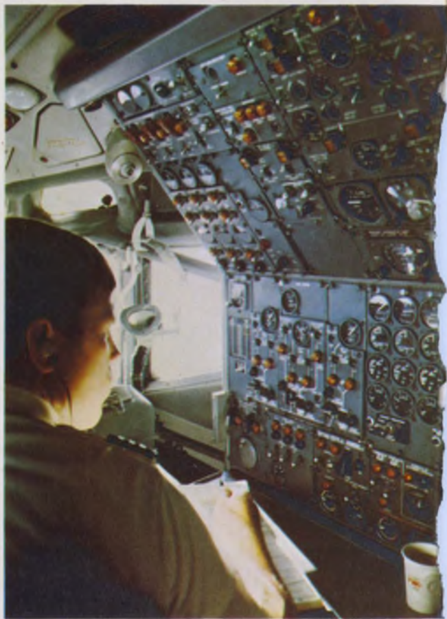
The well-organized flight engineer's controls in this Lockheed 1011 of the Trans World Airlines fleet avoid the sensory overload that could result from large amounts of data on a cluttered panel.
