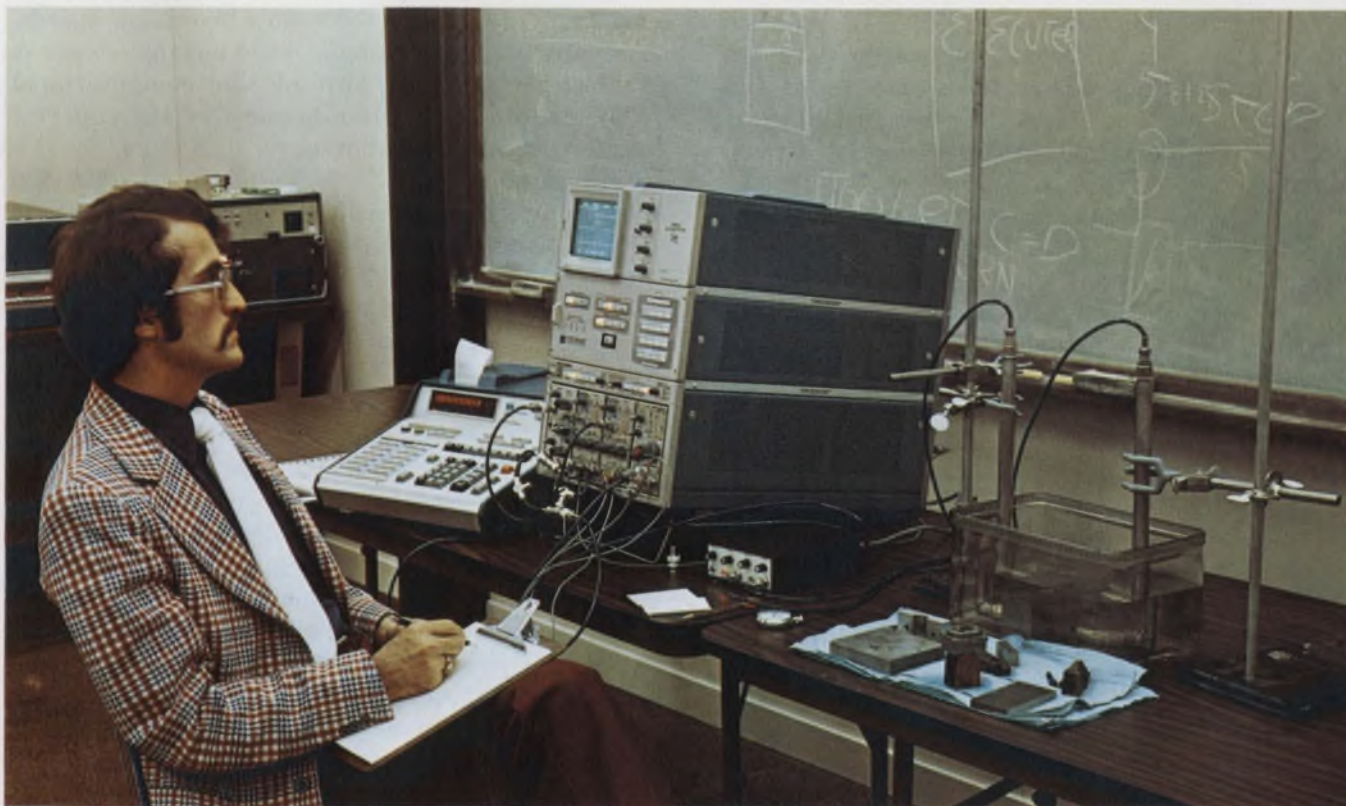
A digital processing oscilloscope and a programmable calculator, by Tektronix, talk to each other a
