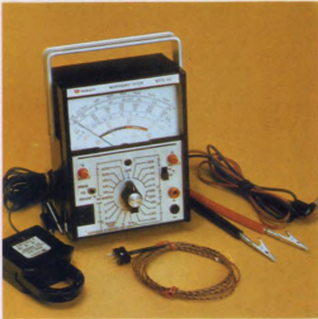
The Triplet Model 615 is a 20,000 ohms-per-volt multi-tester with a -50 to +1500 F thermocouple thermometer. Accuracy is \pm 3\% of full scale.
