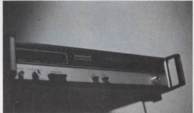
The latest automatic 18-GHz counter costs less than $4000. Standard minimum sensitivities are -20 dBm at 12 GHz and -15 dBm at 18 GHz. The unit, from EIP (Santa Clara, CA) also has a 40-MHz, pk-pk, FM tolerance to 10-MHz modulation.
