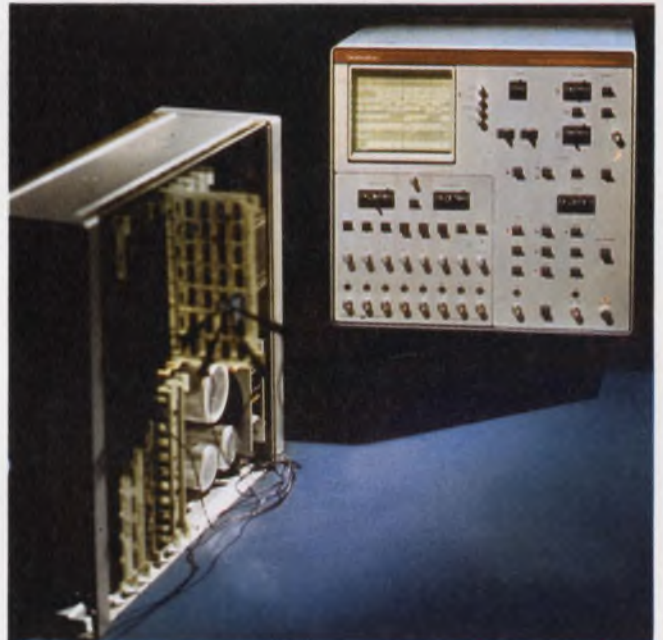
High speed logic can be analyzed with the 8200 logic analyzer from Biomation. It can accept 8 channels of data at a rate of 200 megabits/s.
