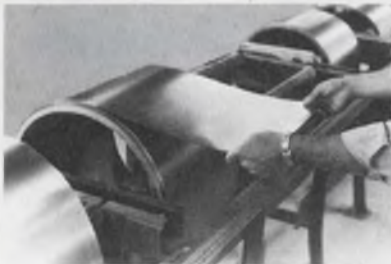
Netic and Co-Netic foil is easily shaped into simple shield configurations.
