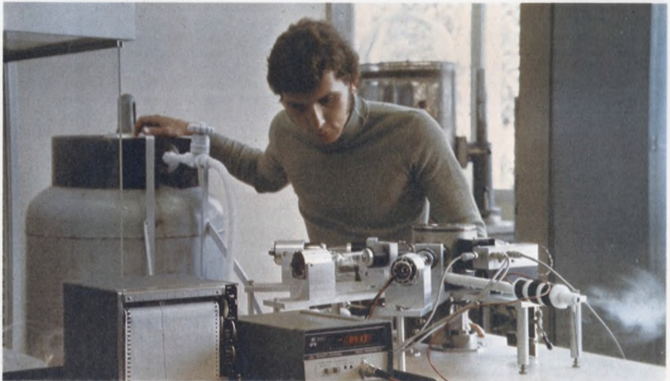
The HP 2801A quartz thermometer (shown with a d/a converter and analog recorder) is a precise laboratory instrument priced at over $3000. Covering the -80 to
