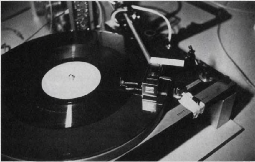
Outer portion of Bogen's magnetic disc contains a thin coating of \text{CrO}_2 , while the inner portion contains grooves that guide the magnetic pickup head.
