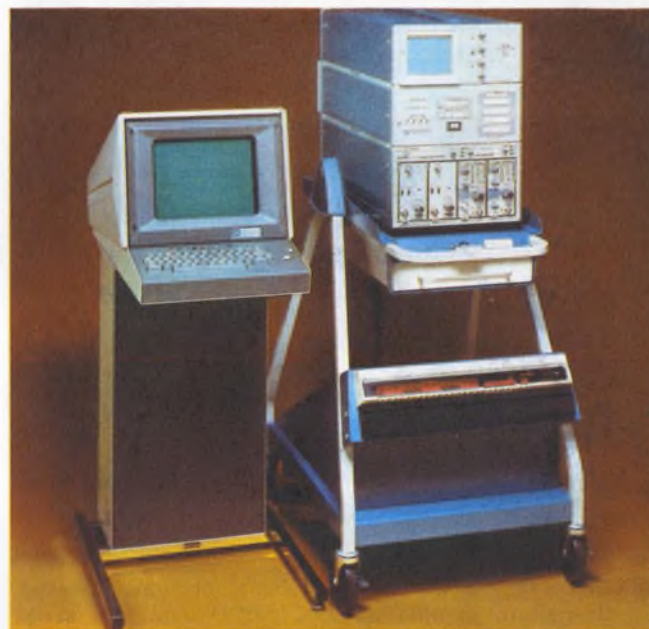
When connected to a 7000 series scope and a PDP-8 computer, the Tektronix digital-processing plug-in, Model 7001, does a multitude of data-acquisition tasks when hooked up to the desired scope plug-ins.
