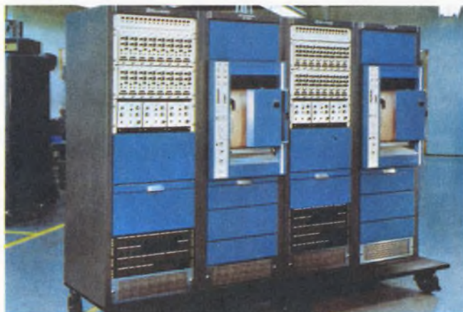
This Bell & Howell data-acquisition system makes possible a variety of applications. The multichannel inputs can be plotted on the X-Y recorders housed in the rack.
