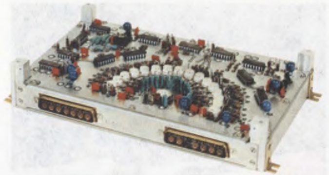
Radial arrangement of components in the Computer Labs Model 7110 a/d converter keeps propagation delays constant between all the converter signal paths. This unit converts 10 bits at 10 MHz.
