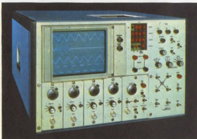
Any or all of four input channels can be displayed by the Macrodyne ERDAC III data-acquisition system. The instrument digitizes and stores incoming analog signals.
