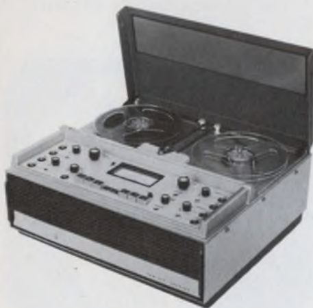
The 3960A recorder uses ¼ in. (0.6 cm) tape or standard 7 in. (17.8 cm) reels.
